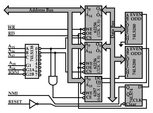
b) (5 pts) BRIEFLY explain how a Non-Maskable Interrupt (NMI) signal is generated using RD, Clk, the parity checker and the 6287 DI/DO pins in the diagram given above.
