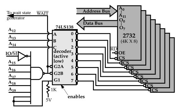
d) (5 pts) Using the information given above, give the address range that the 8 2732s span.
