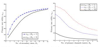
(a) Primary user utility function  $u_{p,j}$  (b) Primary user utility function  $u_{p,j}$ as a function of secondary system size as a function of primary system size  $K_s$ .  $K_p$ .
