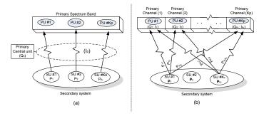
Fig. 1. a) The Centralized Dynamic Spectrum Leasing (C-DSL). b) The Distributed Dynamic Spectrum Leasin (D-DSL)
