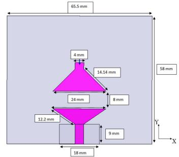
Fig. 5. The "reconfigurable communicating" antenna structure.
