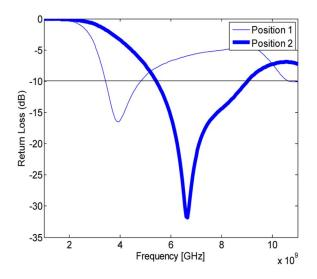
Fig. 7. Frequency tuning for the "reconfigurable communicating" antenna.
