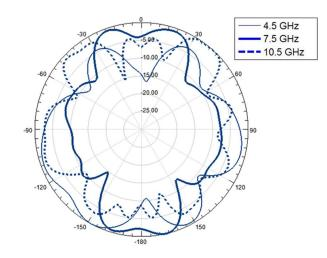
Fig. 4. The normalized antenna radiation pattern for a set of frequencies.
