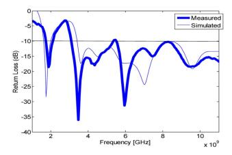
Fig. 11. The "sensing" antenna return loss.
