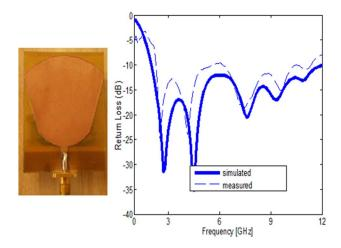
Fig. 1. The antenna structure and its return loss.
