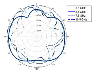
Fig. 14. The normalized antenna radiation pattern.
