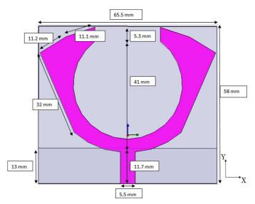
Fig. 2. The "sensing" antenna structure.
