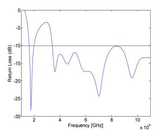
Fig. 3. The return loss for the sensing antenna structure.
