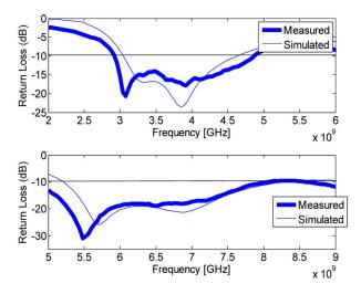
Fig. 12. The "reconfigurable communicating" return loss for both positions.
