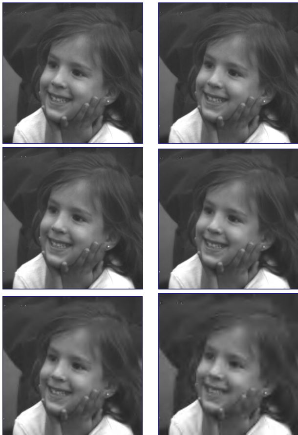
Figure 2. First row: Original and 2 bits/pixel image; Second row: 1 bits/pixel image and 0.5 bits/pixel image Third row: 0.25 bits/pixel image and 0.125 bits/pixel image
