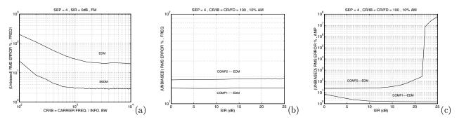
Fig. 2. (a) Effect of CR/IB on EDM frequency demodulation obtained by averaging over FM modulation indices  $\in \{0.1 - 1\}\%$ . (b,c) Effect of SIR on EDM frequency and amplitude demodulation.
