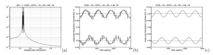
Fig. 1. (a) Fourier spectral magnitude of mixture signal. (b) Angular frequency estimates of the EDM as fractions of  $\pi$ . (c) Frequency estimates of the SEDM, i.e. the estimates in (b) after post-smoothing.
