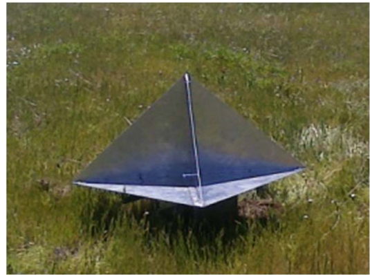
Fig. 15. Experiment I: Vibrating target on the test ground near Julian, CA. The target is an aluminum triangular trihedral with a lateral length of 21 in. The vibration frequency and amplitude were 1.0 Hz and 1.5 cm, respectively.
