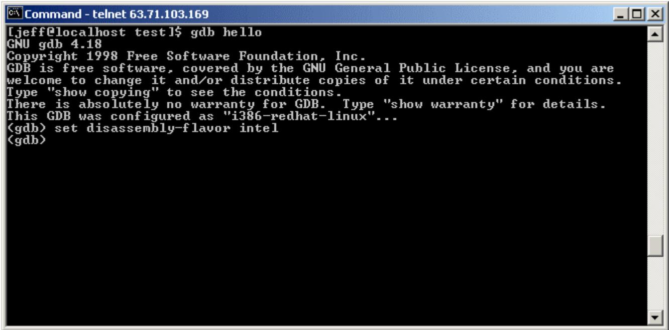
A terminal window titled "Command - telnet 63.71.103.169" showing the output of running 'gdb hello'. The output includes the GNU gdb 4.18 version, copyright information, and license details. The user has entered the command 'set disassembly-flavor intel' to change the default assembly format from AT&T to Intel.
