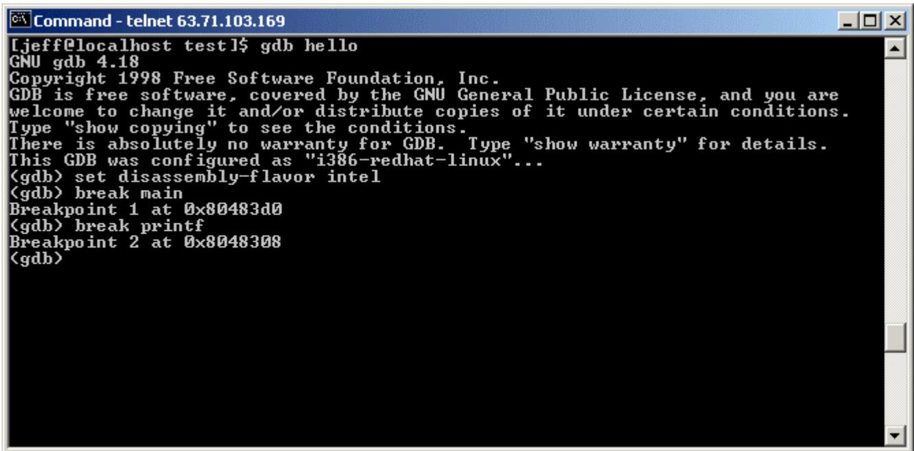
A terminal window titled "Command - telnet 63.71.103.169" showing the continuation of the gdb session. The user has entered 'break main' and 'break printf', which have resulted in two breakpoints being set at memory addresses 0x80483d0 and 0x8048308 respectively.
