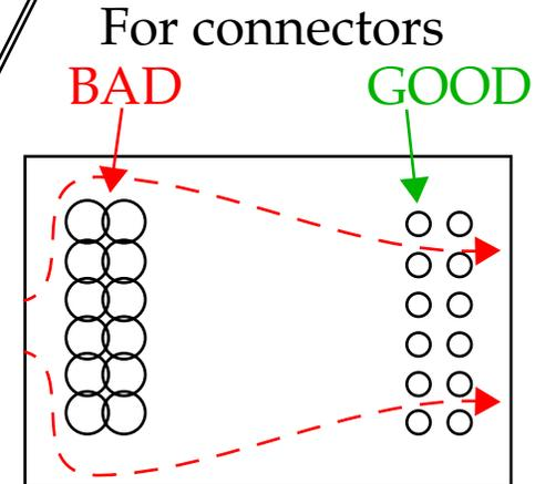
You may be tempted to do this when you run out of room on the regular routing layers and *cram* a trace in on the GND plane.
