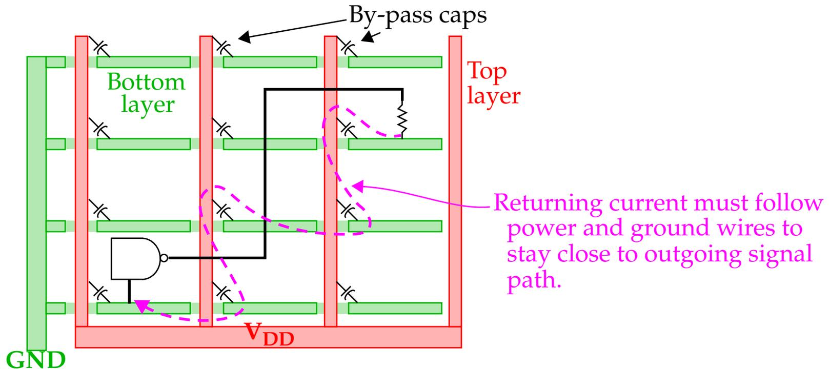
Note that signals are interleaved with the power and GND routing.
