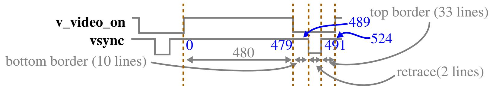
The time unit of the movement is in terms of the horizontal scan lines.
