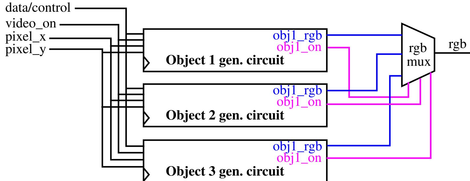
The object generation circuits stores the coordinates of the object and compares them with the current scan location (`pixel_x` and `pixel_y`)
