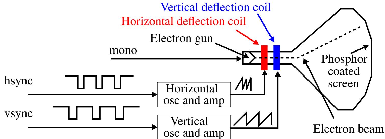
The electron gun generates a focused electron beam that strikes the phosphor screen
