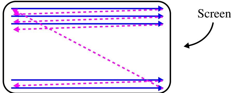
The horz and vert. osc. and amps gen. sawtooth wfms to control the deflection coils
