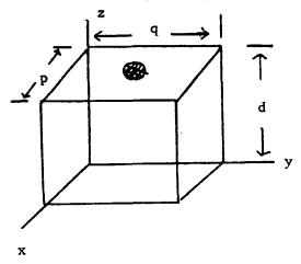
medium of propagation is vacuum and the walls are perfectly conducting.
