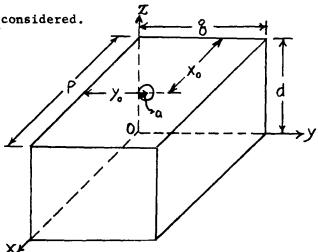
The medium of propagation is assumed to be vacuum and the walls are assumed to be perfectly conducting. The electric field in the cavity then can be written as
