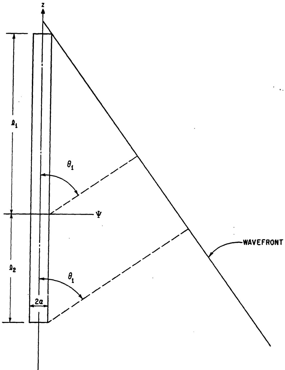
FIGURE 3. FINITE CYLINDRICAL STRUCTURE AND AN INCIDENT ELECTRO-MAGNETIC WAVE.
