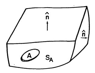
Figure 1. A cavity with an aperture in one of its walls.
