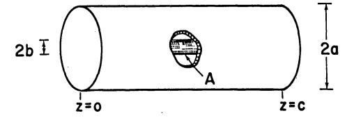
Figure 3. A coaxial cavity with an aperture in the outer conductor.
