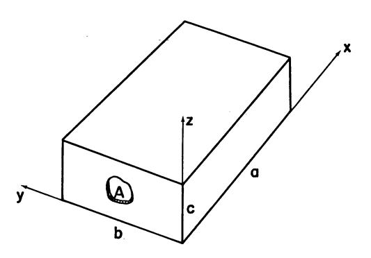
Figure 2. A rectangular cavity with an aperture in one of its walls.
