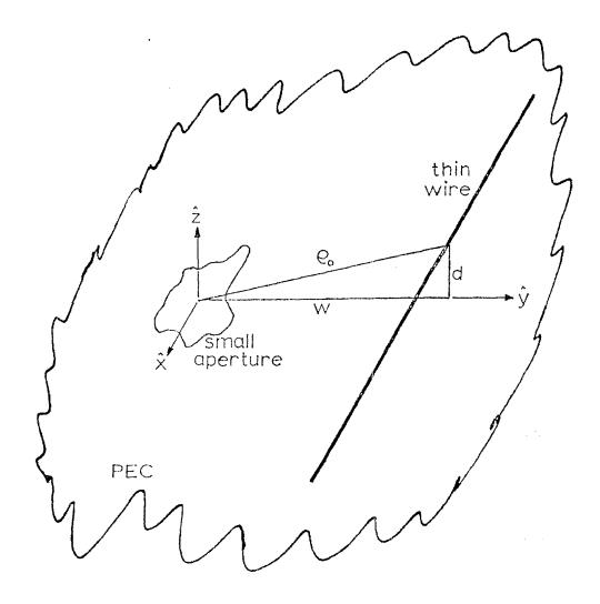
Figure 2. Wire geometry for aperture coupling through a planar perfect electric conductor.
