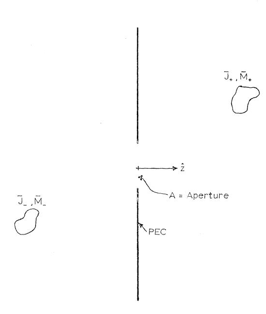
Figure 1. Source locations for aperture coupling through a planar perfect electric conductor.
