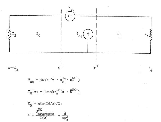
Figure 4. Simplified transmission line model for aperture coupling to a wire behind a planar conductor.
