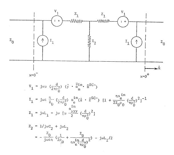
Figure 3. General source and impedance model for the aperture region of a wire behind a planar conductor.
