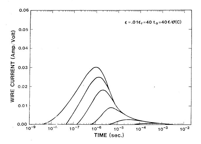
Figure 5c. Wire Currents for  $\sigma$  = 0.01 S/m, and  $\epsilon_{r}$  = 40,  $t_{0}$  = 40 $t_{e}$
