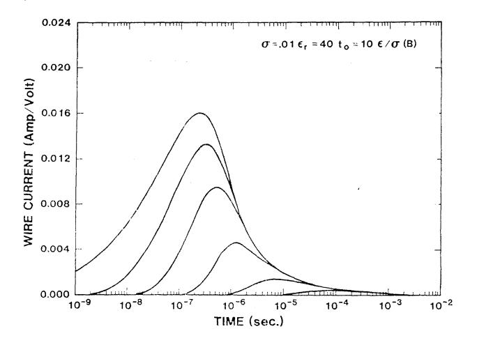
Figure 4b. Wire Currents for  $\sigma$  . 0.01 S/m, and  $\epsilon_{r}$  = 40,  $t_{0}$  = 10te
