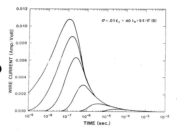
Figure 3b. Wire Currents for  $\sigma$  = 0.01 S/m, and  $\varepsilon_{r}$  = 40,  $t_{0}$  = 5 $t_{e}$
