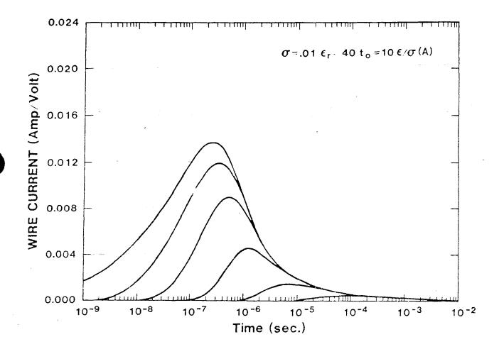
Figure 4a. Wire Currents for  $\sigma = 0.01$  S/m, and  $\epsilon_r = 40$ ,  $t_0 = 10t_e$
