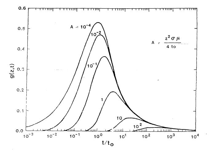
Figure 1. Universal Curves for Wire Currents Due to a Localized Voltage Source. These curves are obtained by a diffusion approximation.
