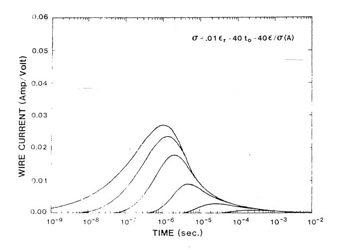
Figure 5a. Wire Currents for  $\sigma$  = 0.01 S/m, and  $\epsilon_r$  = 40,  $t_o$  = 40 $t_e$
