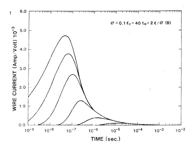
Figure 2b. Wire Currents for  $\sigma = 0.01$  S/m, and  $\epsilon_r = 40$ ,  $t_0 = 2t_e$
