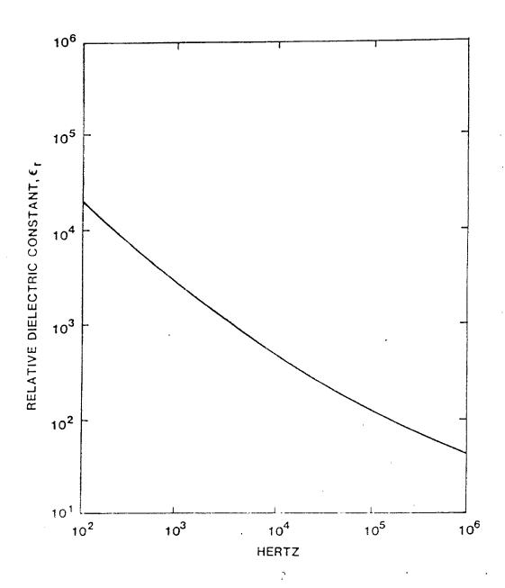
Figure 7. The Relative Dielectric Constant  $\epsilon_{\Gamma}$  Versus Frequency for 10 Percent by Volume of the Water Content
