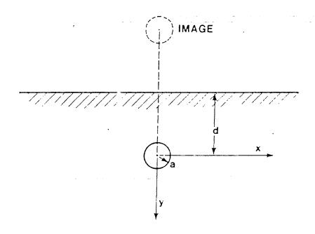
F gure 6b. The Side View of a Buried Wire With Its Image
