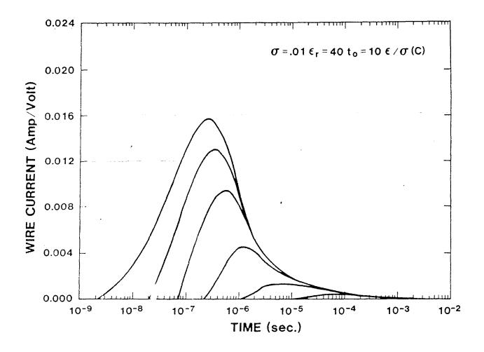
Figure 4c. Wire Currents for  $\sigma$  = 0.01 S/m, and  $\varepsilon_{r}$  = 40,  $t_{0}$  = 10 $t_{e}$
