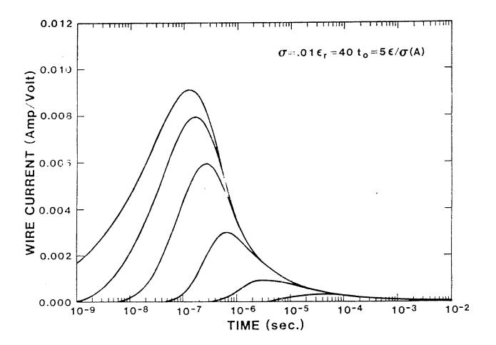
Figure 3a. Wire Currents for  $\sigma = 0.01$  S/m, and  $\epsilon_r = 40$ ,  $t_0 = 5t_e$
