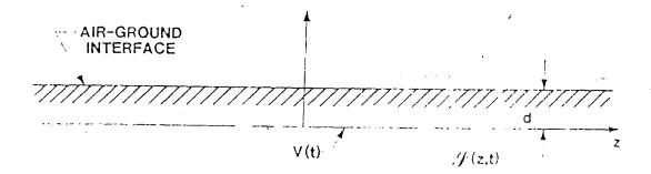
Figure 63. The Geometry of a Buried Wire With an Air Ground Interface
