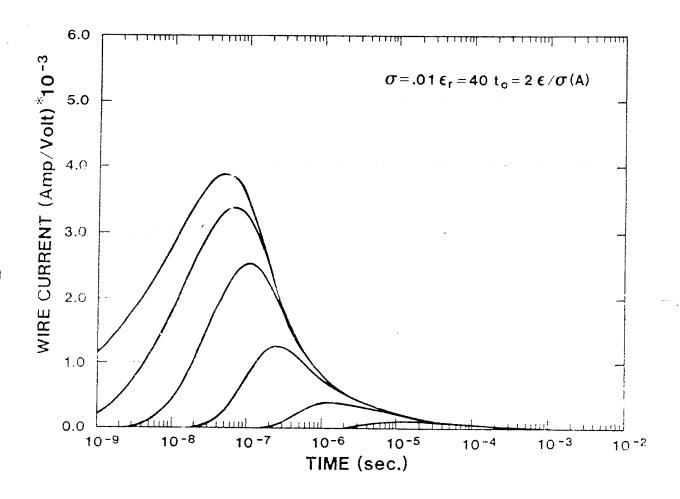
Figure 2a. Wire Currents for  $\sigma$  = 0.01 S/m, and  $\varepsilon_{r}$  = 40,  $t_{0}$  = 2 $t_{e}$
