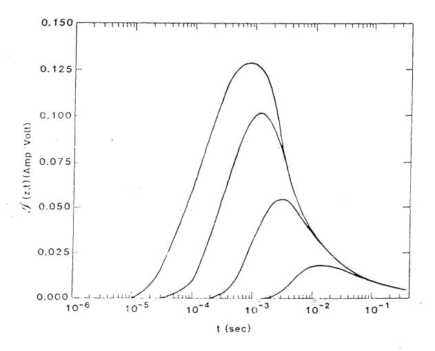
Figure 8. Wire Currents for an Input Voltage at the Gap Given by Equation 15. The locations for the given currents are shown in the figure: from the left z = 100, 316, 1000, and 3160 m. The wire configuration is shown in Figures 6a and 6b.
