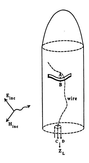
Figure 1. Coupling to a wire inside a slotted cavity.
