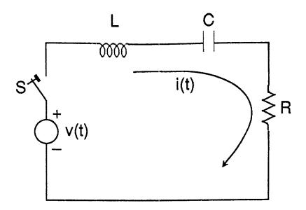
Figure A. Simple L, R, C circuit.
