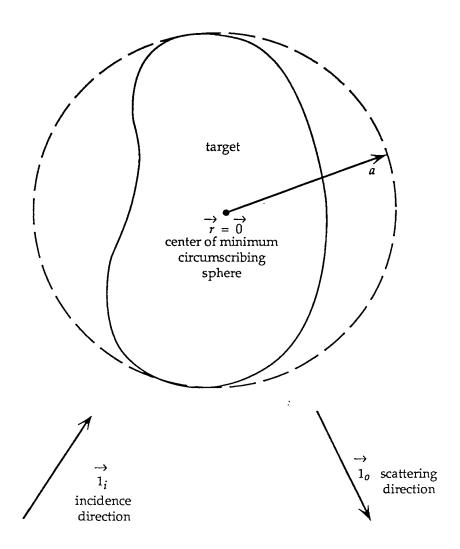
Fig. 1.1 Acoustic and Elastodynamic Scattering from a Target of Finite Linear Dimensions in an Infinite, Homogeneous, Isotropic, Reciprocal, and Linear Medium.
