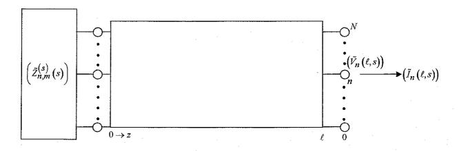
Fig. 2.1 NMTL with Reciprocal Termination at z = 0
