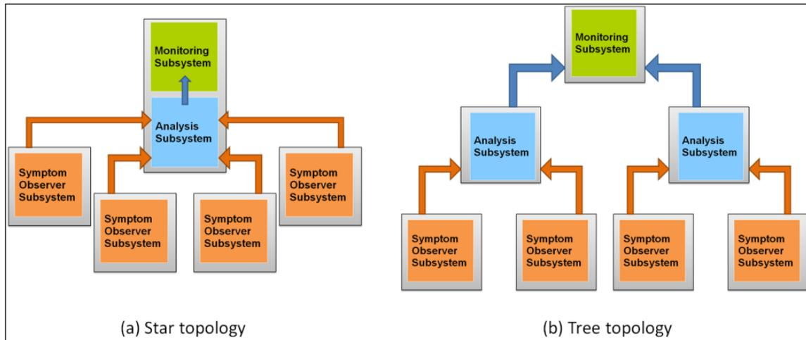
**Fig. 13 : Schematized Star (a) and Tree (b) topologies of a distributed detector integrated in an IT network**
