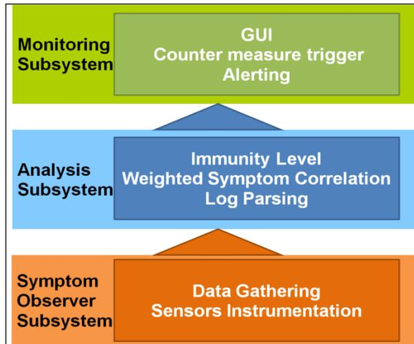
Fig. 12 : Software architecture of the detection system
