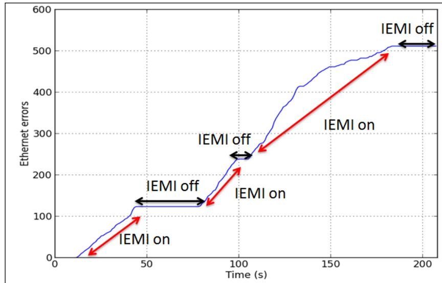
**Fig. 11 : Evolution of errors reported on the Ethernet link during IEMI exposure [21]**
