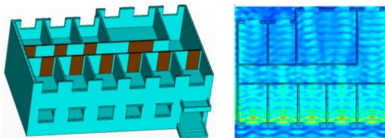
**Fig. 2: Simulation of the EM waves propagation in a building [18]**
