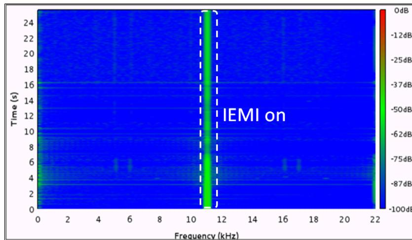
Fig. 8 : Evolution of the noise floor under parasitic EM exposure [21]
