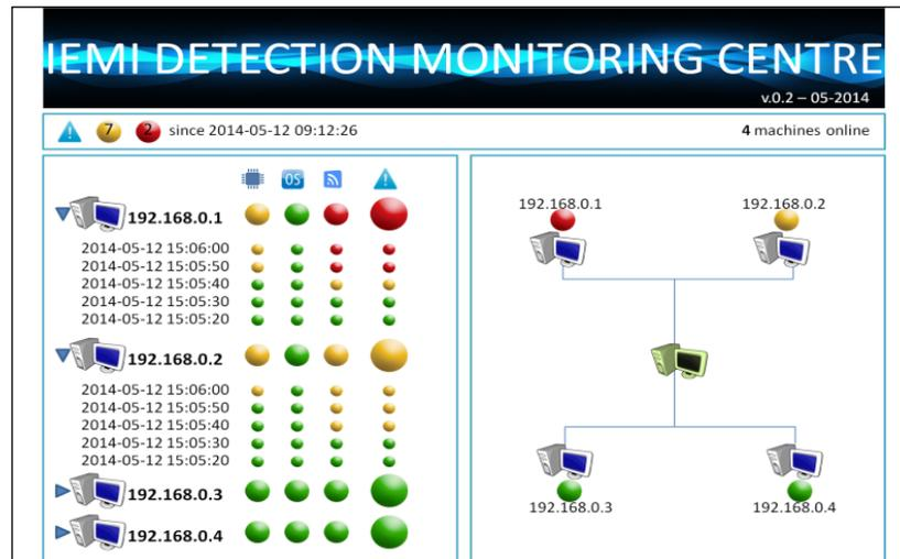
**Fig. 14 : Monitoring interface of the HPEM detection system provided to the operator**
