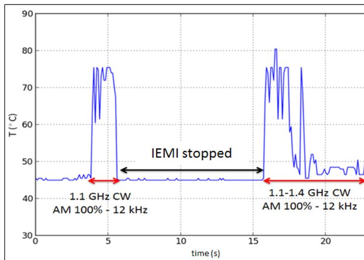
**Fig. 7 : Estimation of the resonating frequency of the temperature sensor for EM coupling maximization**
