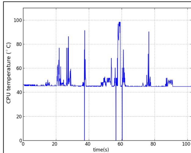
**Fig. 6 : Evolution of the measured temperature under parasitic EM exposure [21]**
