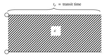
Fig. 3.1 Transmission-Line Capacitive Source
