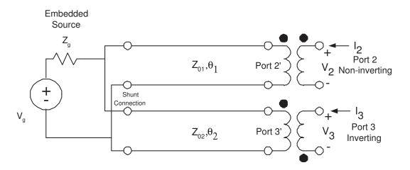
Figure 5: Thévenin Equivalent Model for 3-port consisting of unmatched splitter and invertin transformer.
