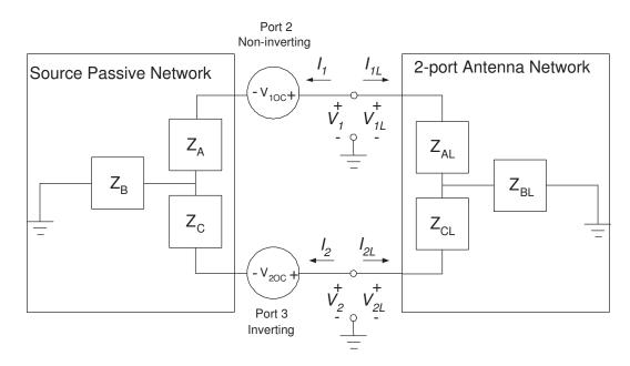
Figure 9: Network connection of 3-port balun model and 2-port antenna model.
