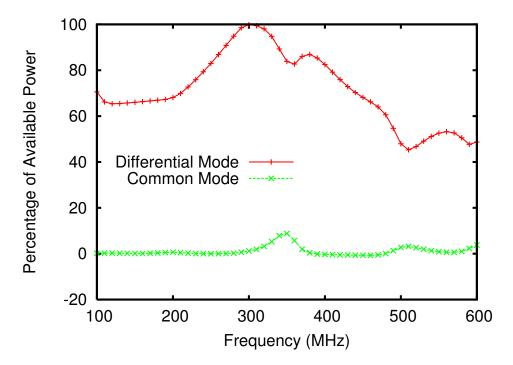
Figure 10: Fraction of available source power carried by differential and common modes. Note that these are modes of the feed system, not radiated power. Some of the power in each mode is delivered to the loads. In particular, most of the common-mode power is dissipated in the loads.
