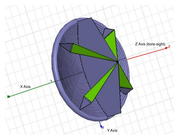
Figure 1: Solid model representing the Farr Research model IRA-3M.
