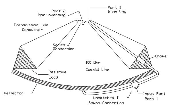
Figure 2: Schematic drawing of feed structure for IRA incorporating 4:1 impedance transforming balun.
