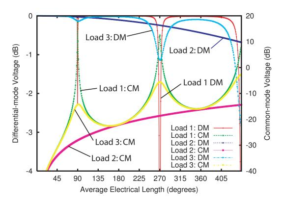
Figure 6: CM and DM Voltages produced by Non-commensurate Balun with +/- 5% physical length difference in constituent transmission lines. The characteristic impedances of the lines are equal with  $Y_{01} = Y_{02} = Y_q/2$ .
