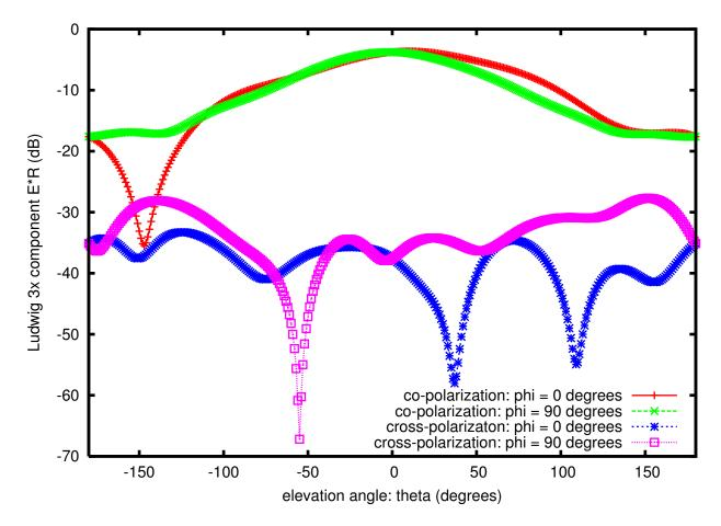
Figure 11: Principal plane radiation patterns for the co- and cross-components of the Ludwig-3 polarization decomposition. The y axis is the Ludwig-3 [12] electric field component multiplied by the radial distance R and normalized to 1 Volt.
