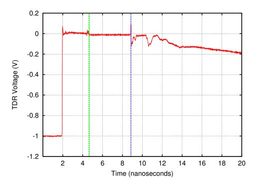
Figure 14: TDR for input of IRA. The green cursor indicates the reflection caused by the shunt splitter; the blue cursor indicates the reflection at the series connection; the interval is 2.1 nanoseconds. The corresponding quarter-wave and half-wave frequencies are approximately 120 and 240 MHz.
