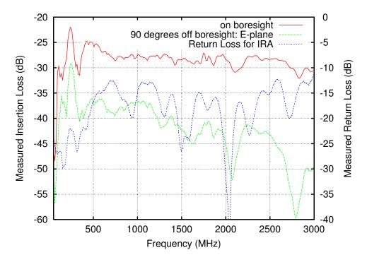
Figure 15: Insertion loss measured between IRA and LPDA augmented with broadband dipole
