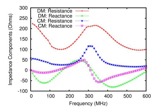
Figure 8: Numerically simulated input impedance at feed point (the junction between the balun and the four feed arms at the focus of the reflector) for equivalent common and differential mode structures. The CM input impedance tends asymptotically to  $\frac{450}{8} = 56.25$  Ohms as the frequency approaches zero while the differential mode input impedance tends asymptotically to  $\frac{450}{2} = 225.0$  Ohms as the frequency approaches zero.
