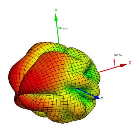
Figure 13: Rendition of the numerically-simulated (with the HFSS finite element simulation program) far-field Ludwig-3 cross-polarized component of the radiation pattern of IRA at 360 MHz. The IRA geometry corresponds to the Farr Research model IRA-3M with a  $\pm 5\%$  disparity in the electrical lengths of the constituent transmission lines of the feed structure. It can be seen that the radiation intensity the *z* direction is very small compared to that generally in the back lobe.
