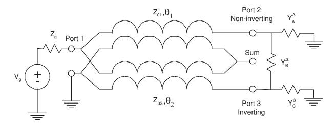
Figure 3: Guanella 4:1 impedance transformer with generalized load. The sum port is equivalent to the sum port of the hybrid described in [3].
