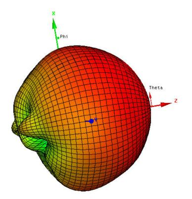
Figure 12: Rendition of the numerically-simulated (with the HFSS finite element simulation program) far-field Ludwig-3 co-polarized component of the radiation pattern of IRA at 360 MHz. The IRA geometry corresponds to the Farr Research model IRA-3M with a  $\pm 5\%$  disparity in the electrical lengths of the constituent transmission lines of the feed structure. It can be seen that the maximum radiation intensity is in the *z* direction.
