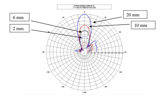
Figure 8. Radiation patterns at 1 GHz, for a range of minor diameters
