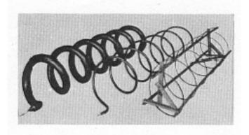
Figure 1. Helical antenna with varying wire radii
