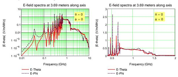
Figure 7. Calculated spectral field at a distance of 3.69m; [500 (V/m)/GHz]
