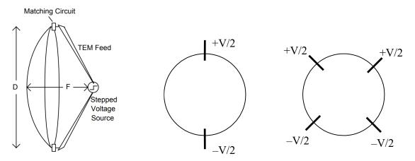
Figure 1. Sketch of a 2-arm IRA (left and center) and a 4-arm IRA (right).
