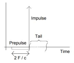
Figure A-1. Sketch of the impulse response of an IRA.
