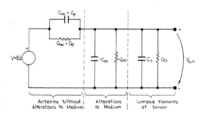
Fig. 5 Equivalent Circuit for Parallel Plate Sensor
