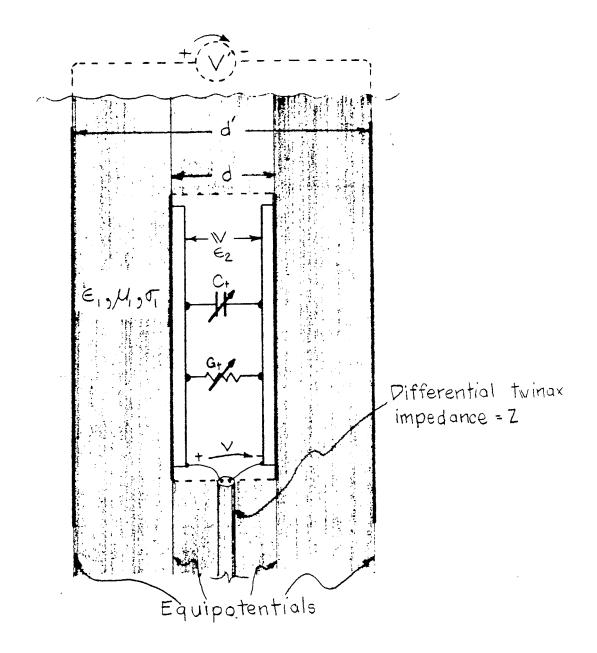
Fig. 4 Calibration System for Matching Sensor to Medium.
