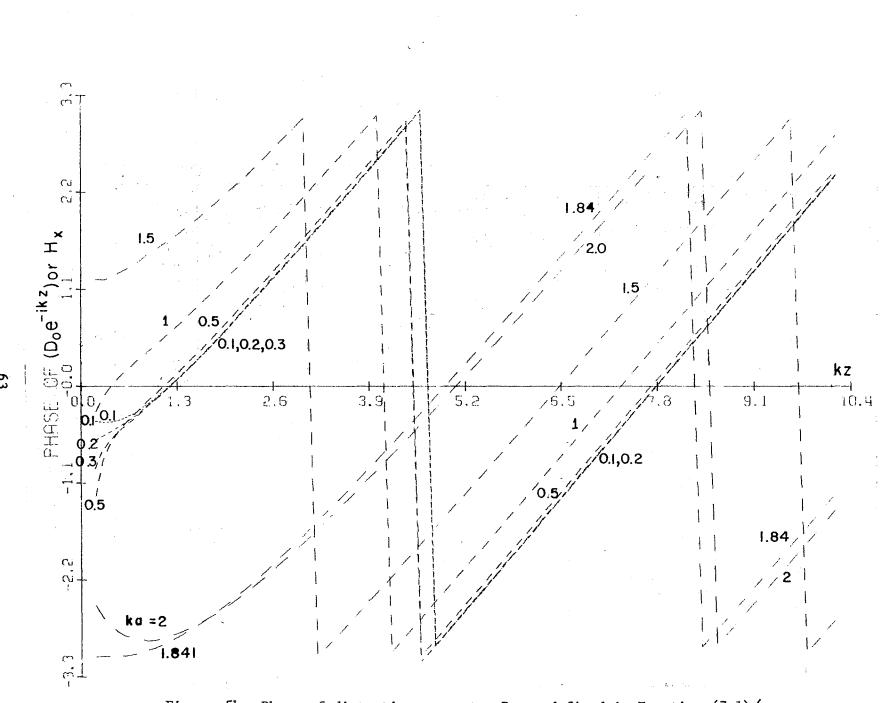
Figure 5b. Phase of distortion parameter D as defined in Equation (7.1), (or that of the scattered field H ) versus kz for a given ka
