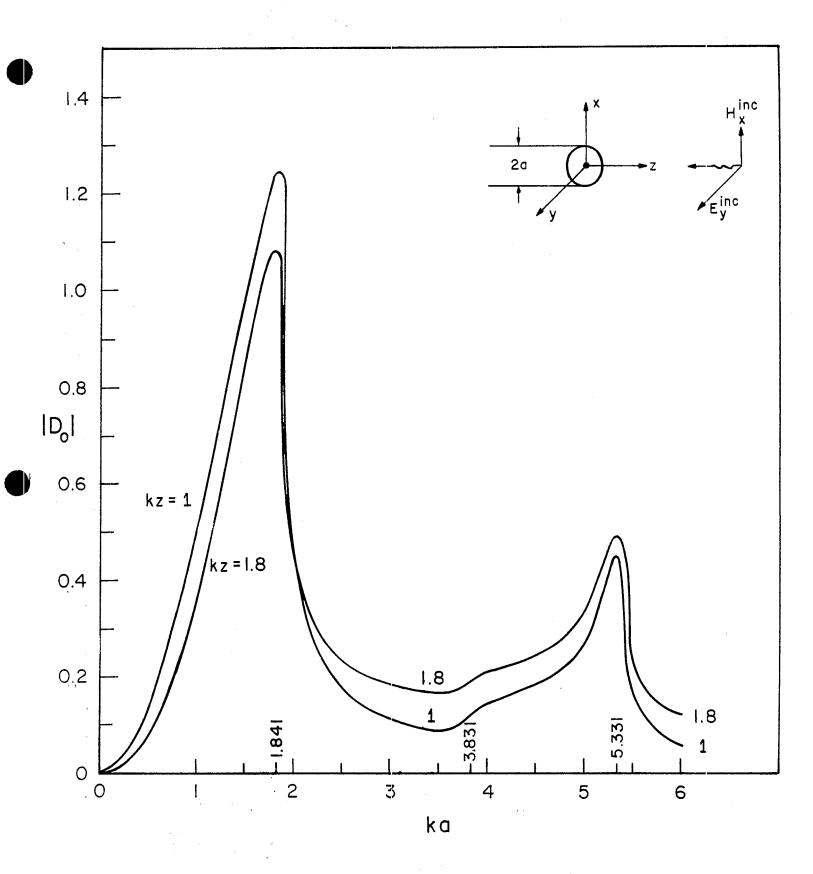
Figure 4. Absolute value of distortion parameter D defined in Equation (7.1) (or the scattered H ) versus ka for a given kz
