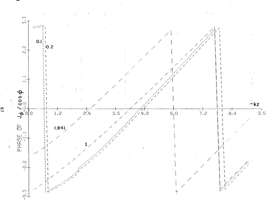
Figure 8b. Phase of the circumferential current  $J_{\varphi}$  versus kz for a given ka
