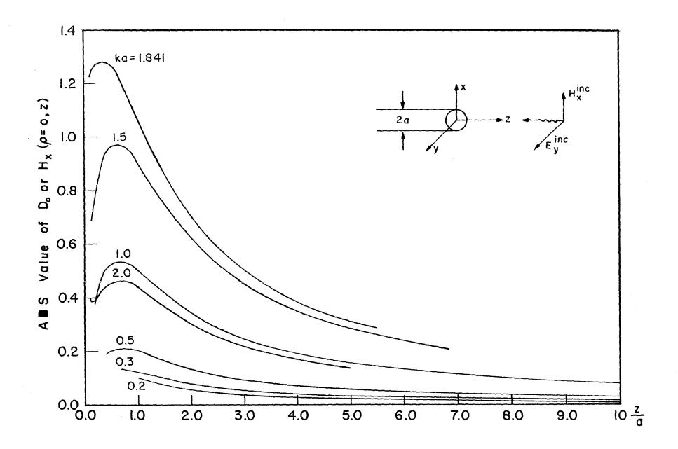
Figure 6. Absolute value of distortion parameter D as defined in Equation (7.1) versus z/a for given ka
