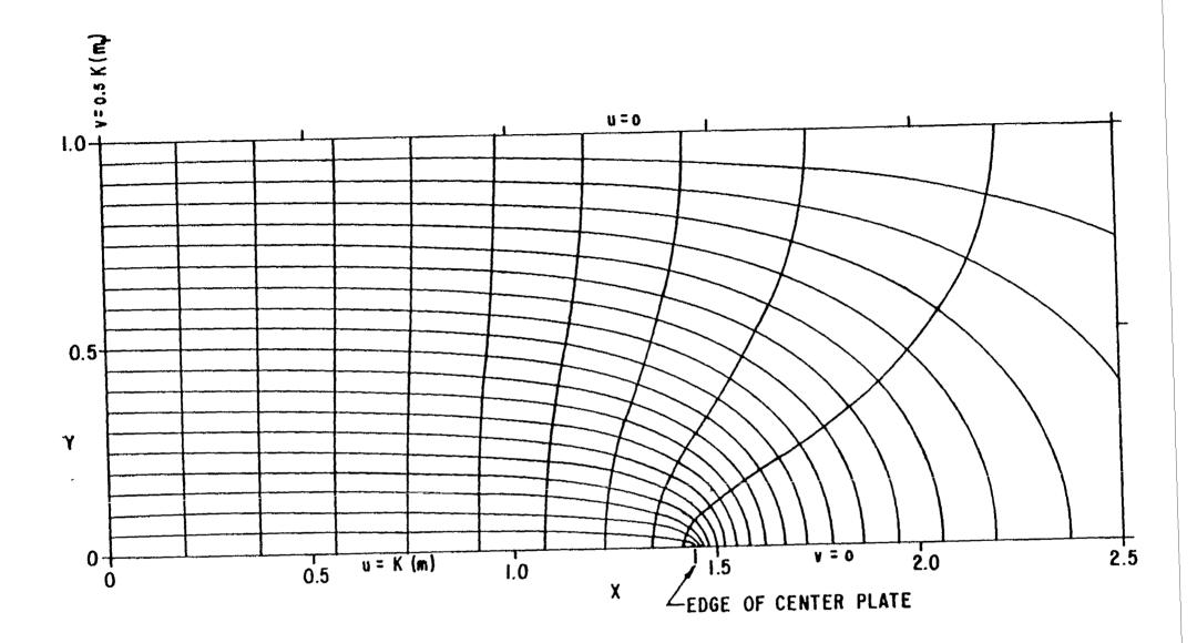
FIGURE 5. FIELD AND POTENTIAL DISTRIBUTION FOR FINITE CENTER CONDUCTOR IN INFINITE THREE CONDUCTOR PARALLEL-PLATE TRANSMISSION LINE: 50 D
