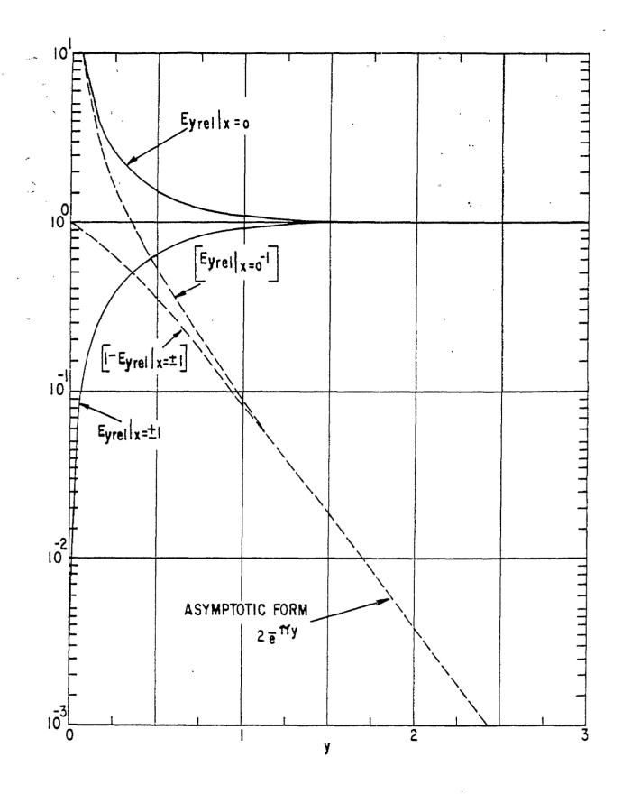
FIGURE 18. NORMALIZED FIELD DISTRIBUTION FOR WIRE GRID TERMINATING EQUAL AND OPPOSITE UNIFORM FIELDS ON BOTH SIDES OF GRID 36
