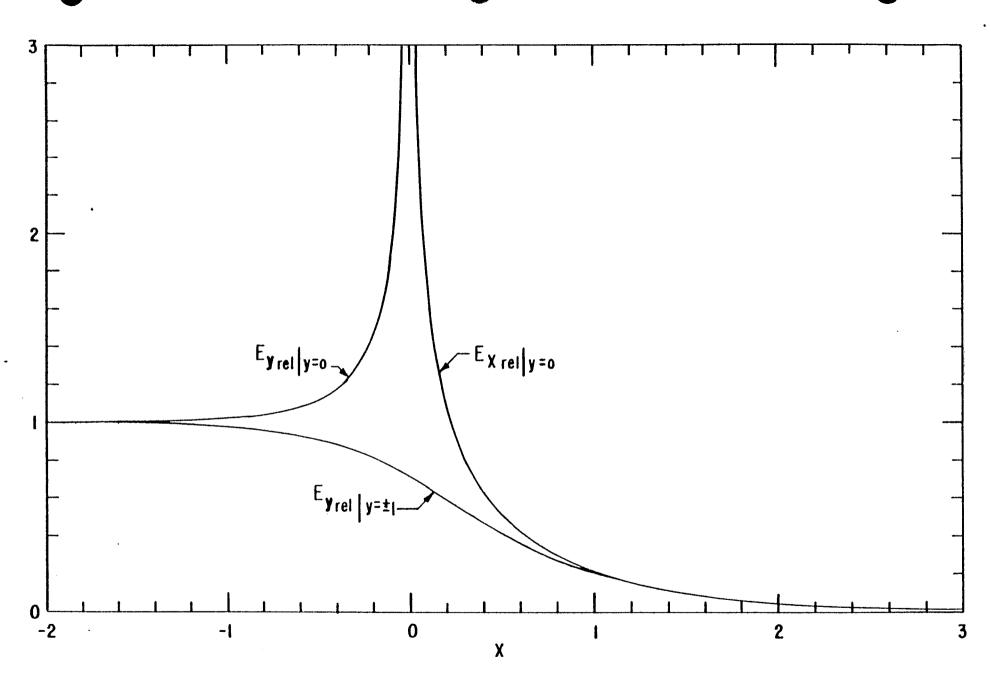
FIGURE 3. NORMALIZED FIELD DISTRIBUTION WITH SEMI-INFINITE CENTER CONDUCTOR IN INFINITE THREE CONDUCTOR PARALLEL PLATE TRANSMISSION LINE
