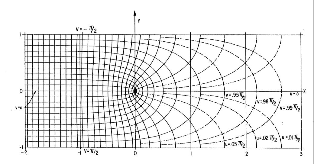
FIGURE 2. FIELD AND POTENTIAL DISTRIBUTION WITH SEMI-INFINITE CENTER CONDUCTOR IN INFINITE THREE CONDUCTOR PARALLEL-PLATE TRANSMISSION LINE In figure 2 the equipotentials and magnetic field lines are given by constant v and the electric field lines by constant u. Rewriting the conformal transformation as
