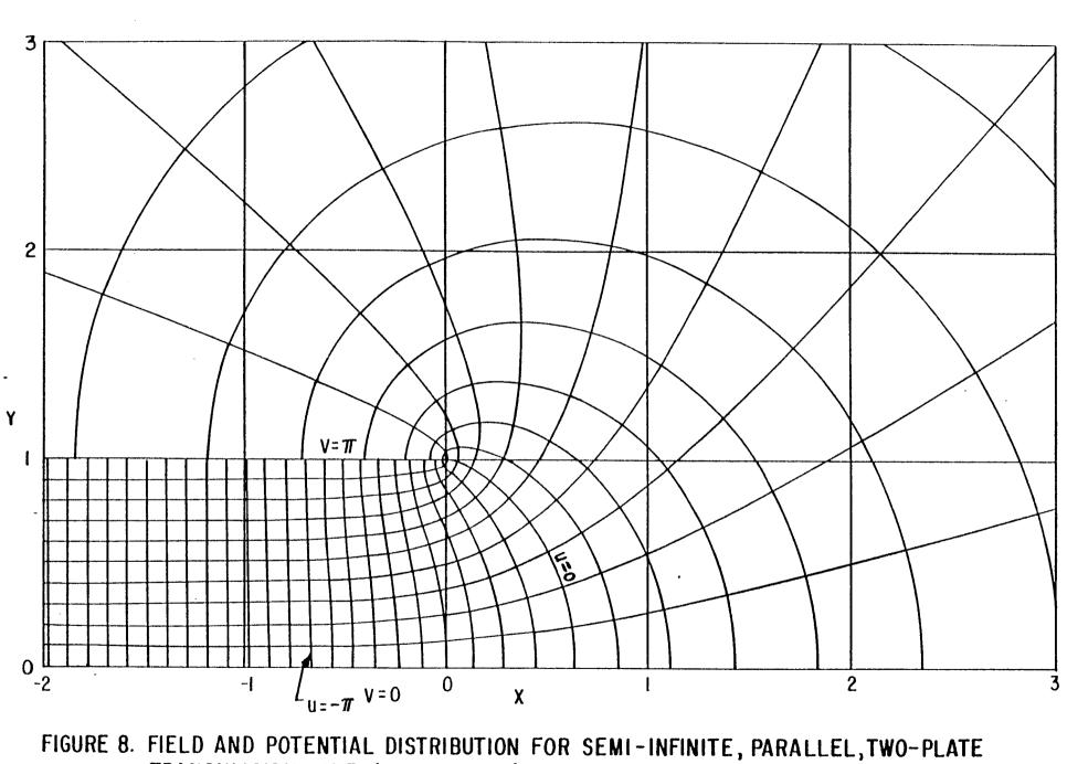
FIGURE 8. FIELD AND POTENTIAL DISTRIBUTION FOR SEMI-INFINITE, PARALLEL, TWO-PLATE TRANSMISSION LINE (UPPER HALF) 17 First calculate the field distribution along the plane of symmetry (y = 0, v = 0). Here we have
