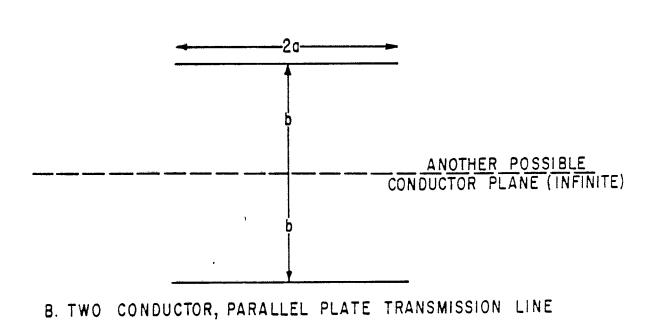
FIGURE I. SYMMETRICAL, PARALLEL PLATE TRANSMISSION LINES
