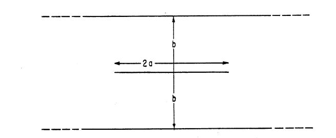
A. INFINITE OUTER PLATES, THREE CONDUCTOR, PARALLEL PLATE TRANSMISSION LINE
