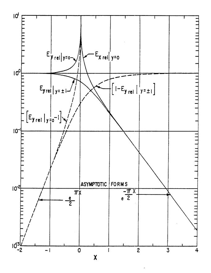
FIGURE 4. NORMALIZED FIELD DISTRIBUTION WITH SEMI-INFINITE CENTER CONDUCTOR IN INFINITE THREE CONDUCTOR PARALLEL PLATE TRANSMISSION LINE 8
