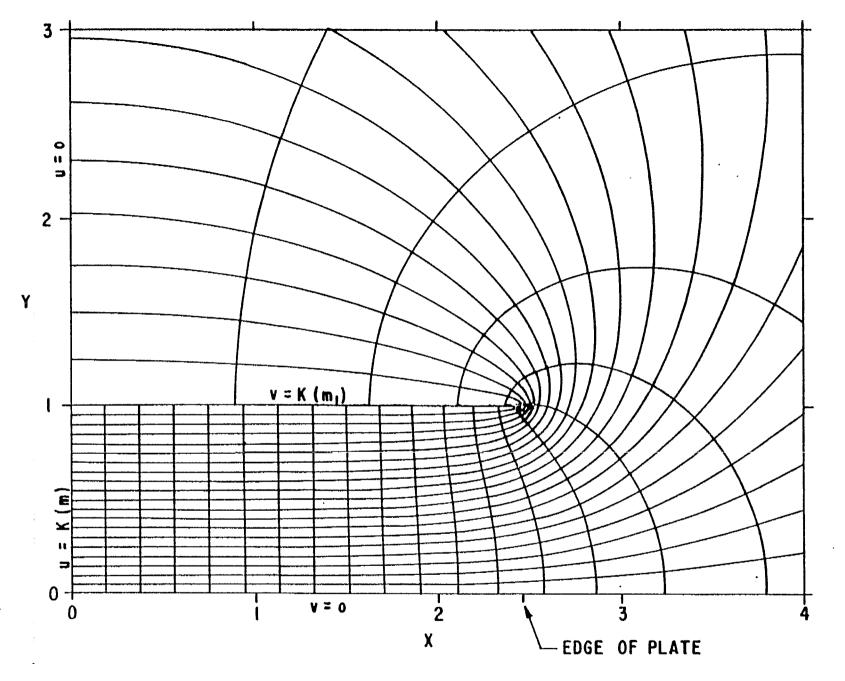
FIGURE II. FIELD AND POTENTIAL DISTRIBUTION FOR PARALLEL, TWO-PLATE TRANSMISSION LINE: 100 A
