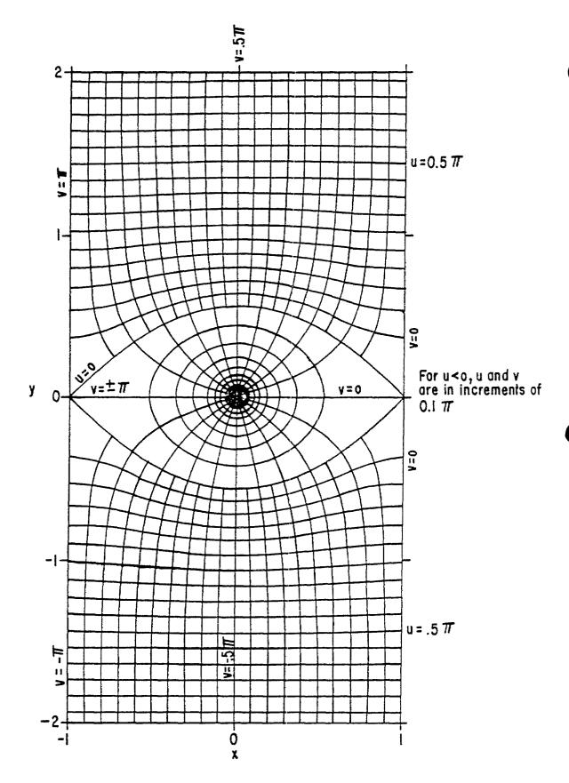
FIGURE 17. WIRE GRID (ONE CELL) TERMINATING EQUAL AND OPPOSITE UNIFORM FIELDS ON BOTH SIDES OF GRID
