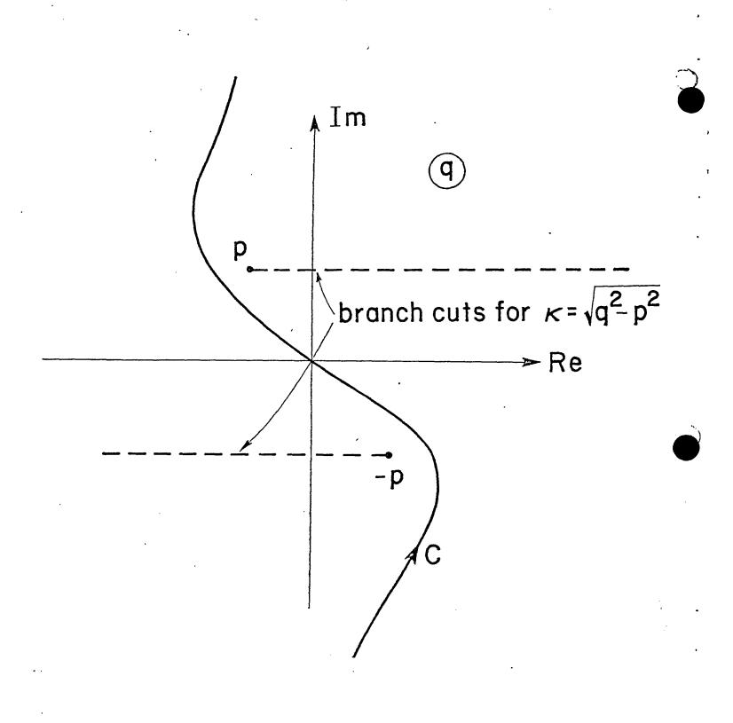
Figure 3. The path of integration C in the inverse . Laplace transform integral.
