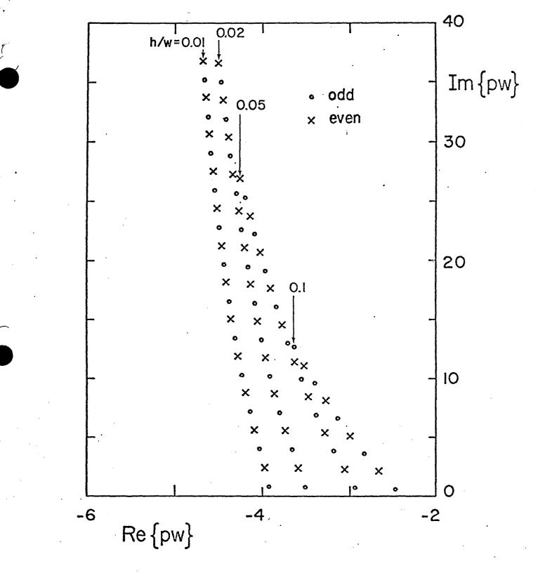
Figure 6. The roots of (70) and (71). Roots such that |ph| << 1are the transverse propagation constants for the antisymmetric TM modes  $(p'_{a,n})$ .
