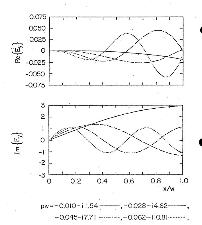
Figure 8a. Transverse variation of the E field component of the four lowest odd antisymmetric TE modes.
