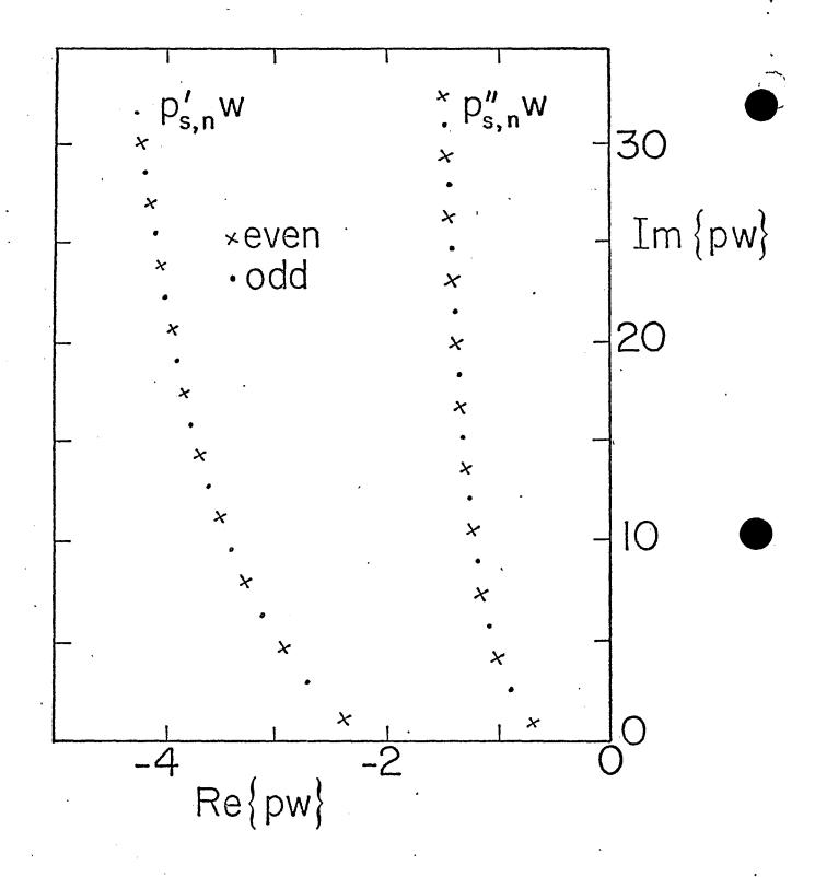
Figure 5. The transverse propagation constants for the symmetric TM modes  $(p'_{s,n})$  and the symmetric TE modes  $(p''_{s,n})$ .
