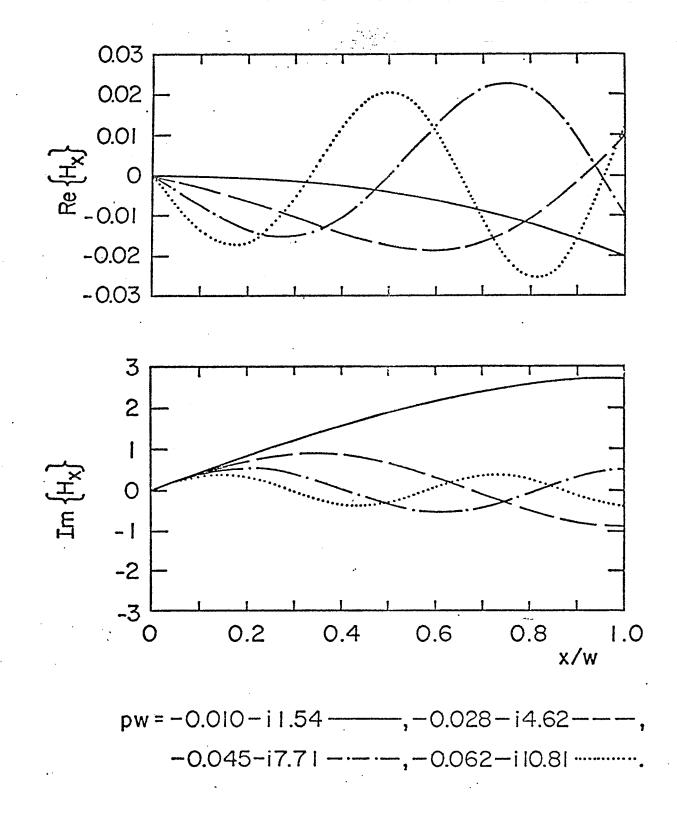
Figure 8b. Transverse variation of the  $H_{x}$  field component of the four lowest odd antisymmetric TE modes.
