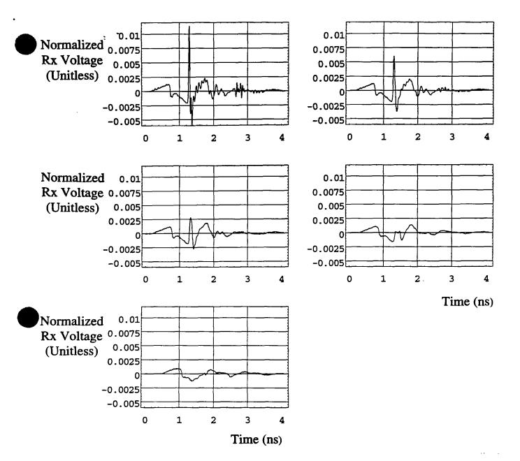
Figure 4.4 (a). E-plane received voltage, after filtering and normalization. Waveforms are at 0, 5, 10, 20 and 40 degrees off boresight.
