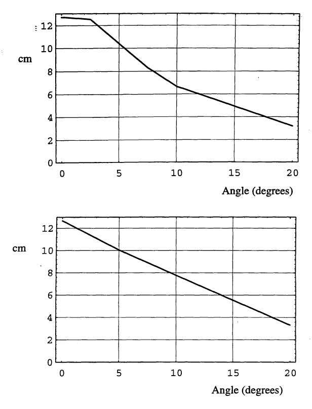
Figure 9.2. Gain of the 23 cm (9-inch) reflector IRA plotted as a function of angle off-boresight in the E-plane (top and in the H-plane (bottom). Here gain is as defined in Equation 5.1 for 50 ps risetime step excitation.
