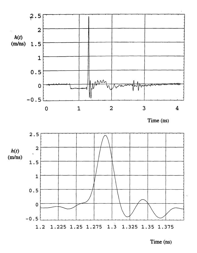
Figure 4.7 Boresight h(t), entire waveform (top) and a closeup of the impulse (bottom).
