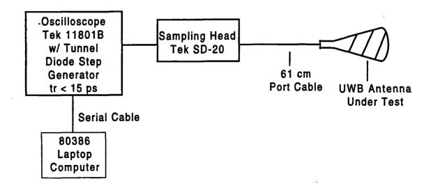
Figure 5.3. Experimental configuration for TDR measurements.
