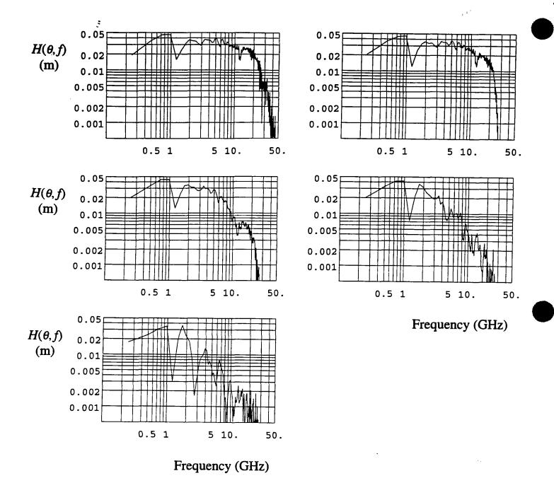
Figure 4.9(b) H-plane  $H(\theta, f)$  at 0, 5, 10, 20, and 40 degrees off-boresight.
