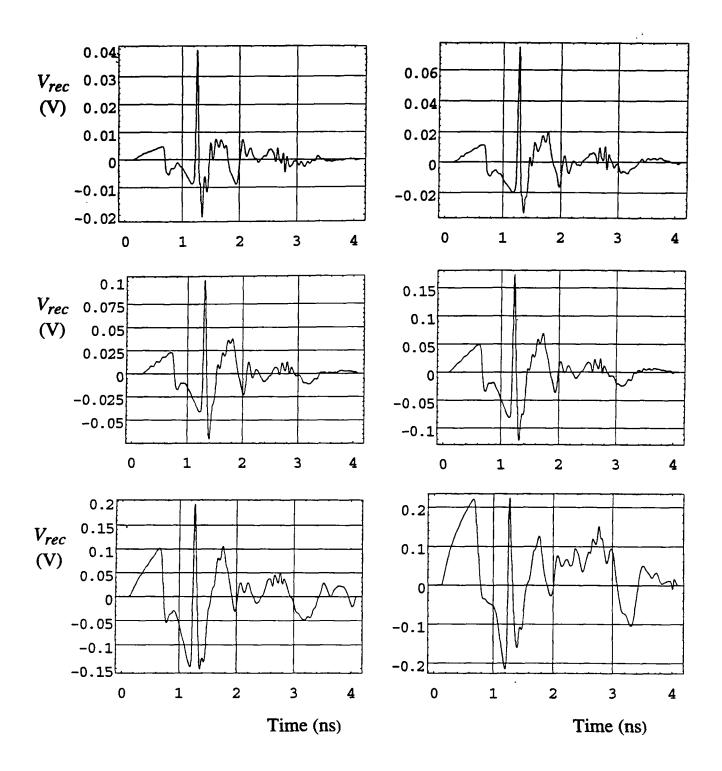
Figure 5.5. Received voltage in the two-antenna measurement, as a function of antenna separation. The distances were 5.66, 2.87, 1.45, 0.71, 0.36, and 0.18 meters.
