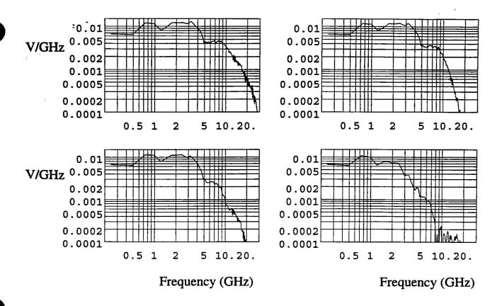
Figure 8.3(b). H-Plane scan, filtered but unnormalized, in the frequency domain. Waveforms are at 0, 5, 10, and 20 degrees off boresight
