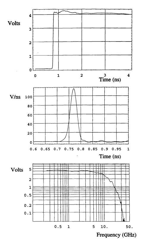
Figure 8.1. The system excitation response (incident voltage and cabling) (top), its derivative after filtering (middle) and its unfiltered frequency spectrum (bottom).
