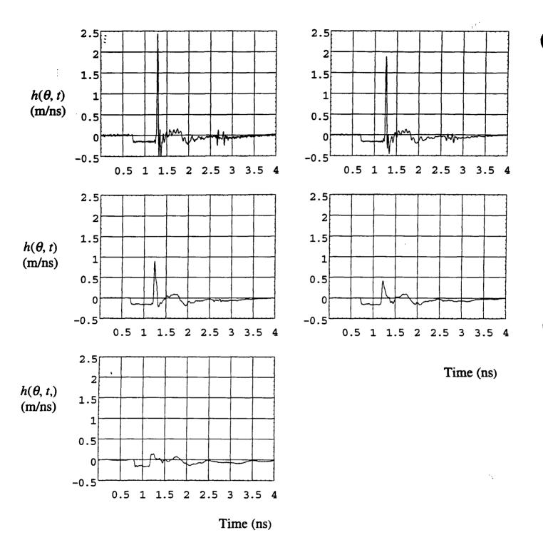
Figure 4.8(b) H-plane  $h(\theta, t)$  at 0, 5, 10, 20, and 40 degrees off-boresight.
