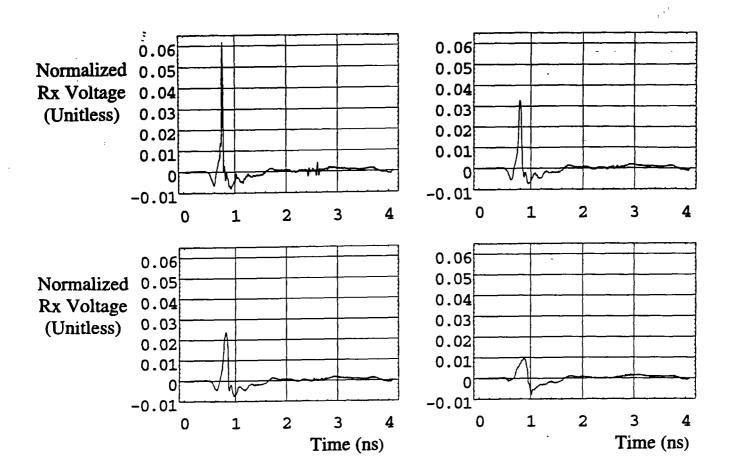
Figure 8.4 (c). H-plane received voltage, after filtering and normalization. Waveforms are at 0, 5, 10, and 20 degrees off boresight.
