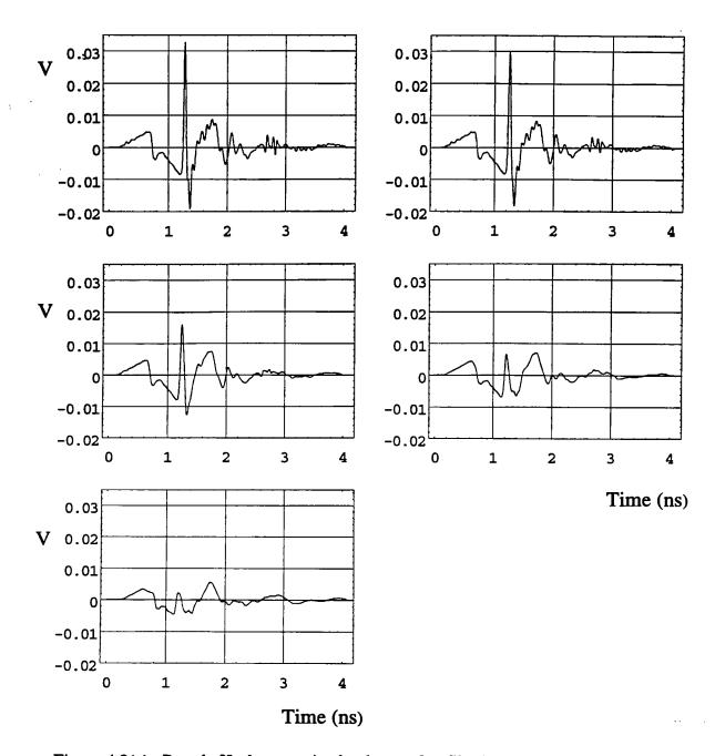
Figure 4.2(c). Pseudo H-plane received voltage, after filtering. Waveforms are at 0, 5, 10, 20 and 40 degrees off boresight
