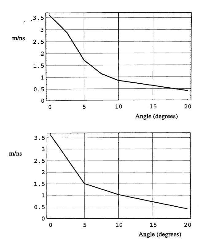
Figure 9.1. Gain of the 23 cm (9-inch) reflector IRA plotted as a function of angle off-boresight in the E-plane (top) and in the H-plane (bottom). Here gain is used in the peak h(t) sense, with perfect step excitation.
