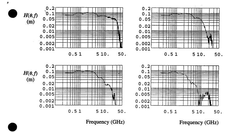
Figure 8.9(b) H-plane  $H(\theta, f)$  at 0, 5, 10, and 20 degrees off-boresight.
