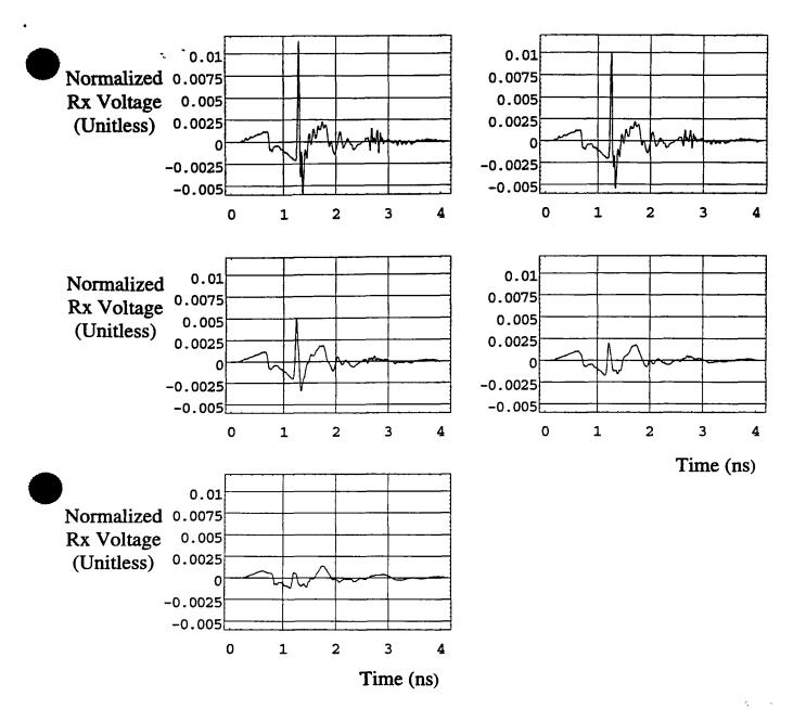
Figure 4.4 (c). Pseudo H-plane received voltage, after filtering and normalization. Waveforms are at 0, 5, 10, 20 and 40 degrees off boresight.
