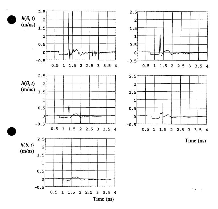
Figure 4.8(a) E-plane  $h(\theta, t)$  at 0, 5, 10, 20, and 40 degrees off-boresight.
