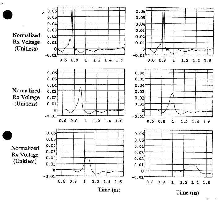
Figure 8.4 (b). Closeup of the peaks in Figure 8.4 (a).
