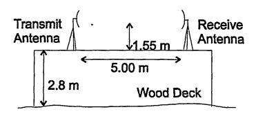
Figure 7.1. The physical layout of the two antennas for the lens IRA measurements.
