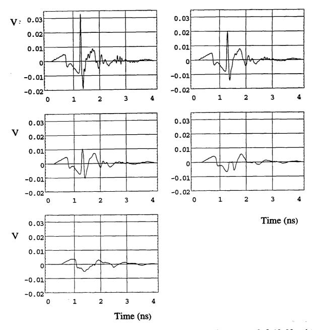
Figure 4.2(a). E-plane received voltage, after filtering. Waveforms are at 0, 5, 10, 20 and 40 degrees off boresight
