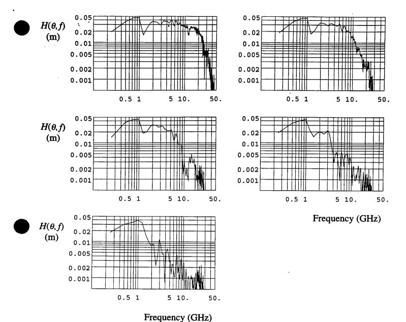
Figure 4.9(a) E-plane  $H(\theta, f)$  at 0, 5, 10, 20, and 40 degrees off-boresight.
