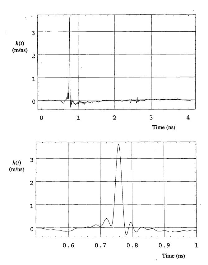
Figure 8.7 Boresight h(t), entire waveform (top) and a closeup of the impulse (bottom).
