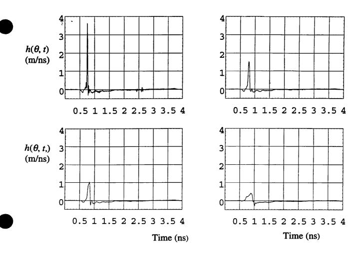
Figure 8.8(b) H-plane  $h(\theta, t)$  at 0, 5, 10, and 20 degrees off-boresight.
