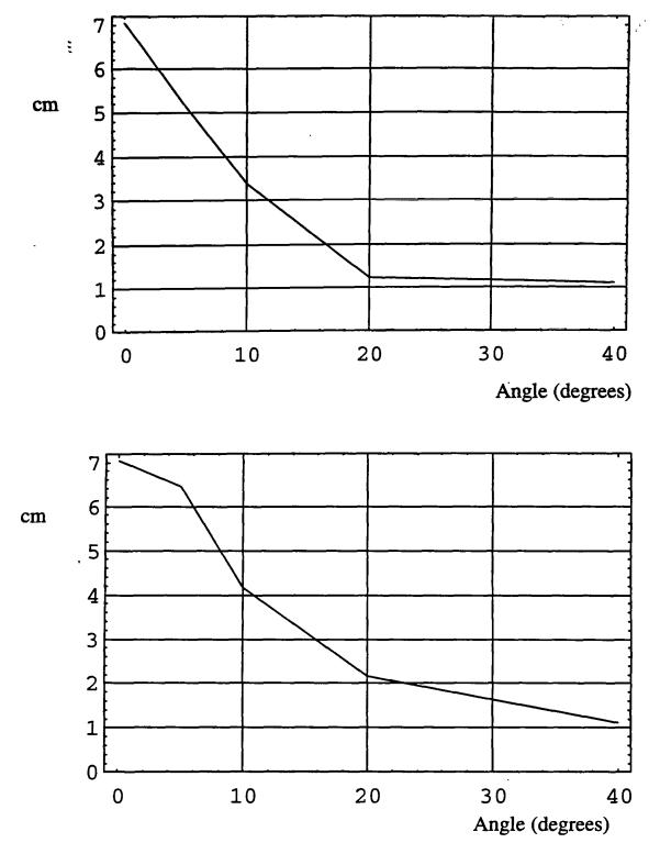
Figure 5.2. Gain of the 23 cm (9 in) reflector IRA plotted as a function of angle off-boresight in the E-plane (top and in the pseudo H-plane (bottom). Here gain is as defined in Equation 5.1.
