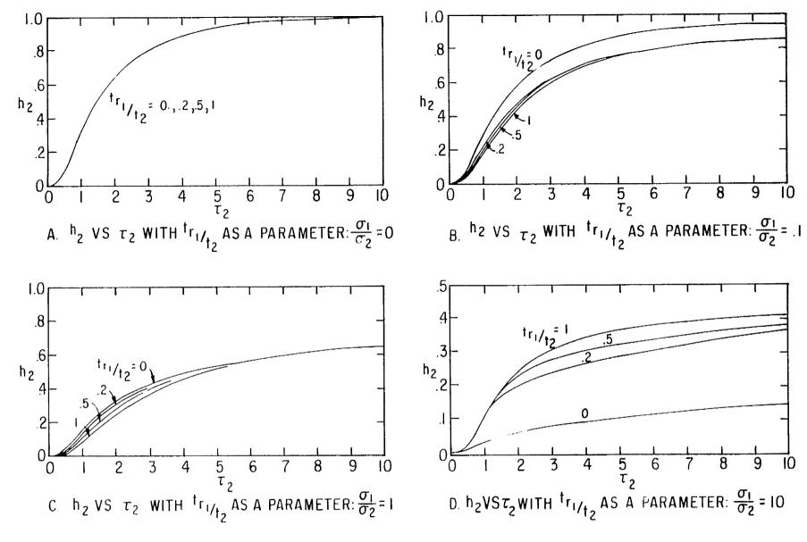
FIGURE 6. MAGNETIC FIELD PULSE SHAPE ON TRANSMISSION LINE:  $\epsilon_{r_1} = 1$ ,  $\epsilon_{r_2} = 10$ ,  $p_5 = 0$
