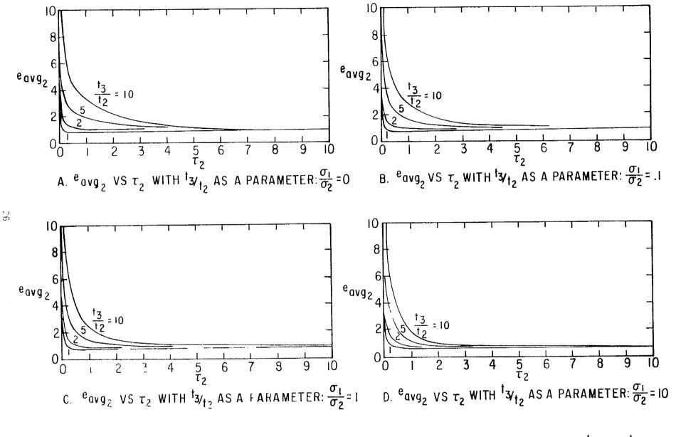
FIGURE 4. AVERAGE VERTICAL ELECTRIC FIELD PULSE SHAPE ON TRANSMISSION LINE: tri/t2 = tr2/t2=0
