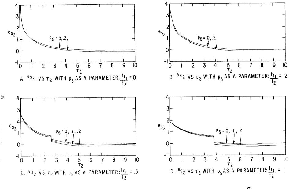
FIGURE 16. HORIZONTAL ELECTRIC FIELD PULSE SHAPE ON TRANSMISSION LINE:  $\frac{\sigma_1}{\sigma_2} = 0$ ,  $\epsilon_{r_1} = 10$
