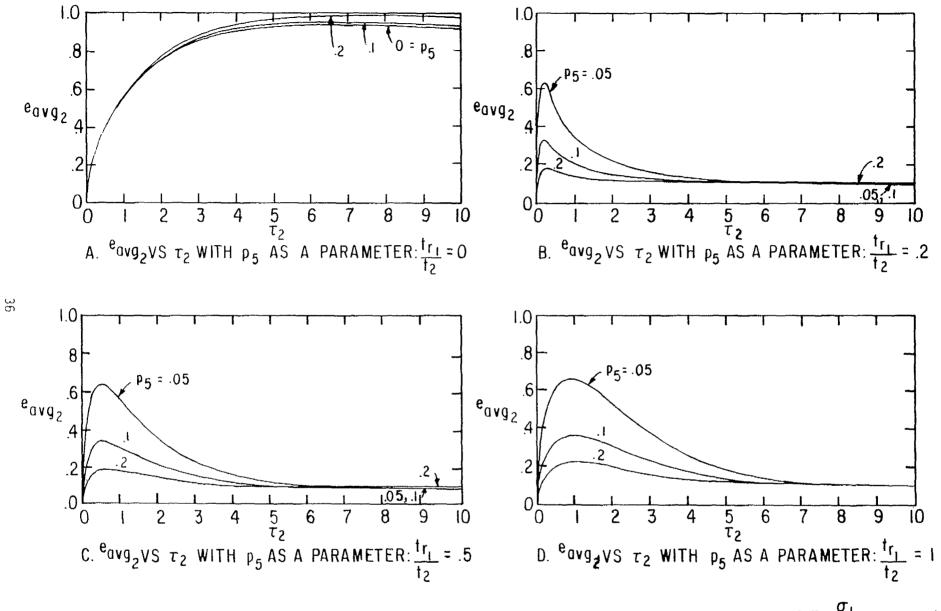
FIGURE 14. AVERAGE VERTICAL ELECTRIC FIELD PULSE SHAFE ON TRANSMISSION LINE:  $\frac{\sigma_1}{\sigma_2} = 0, \epsilon_{r_1} = 1$
