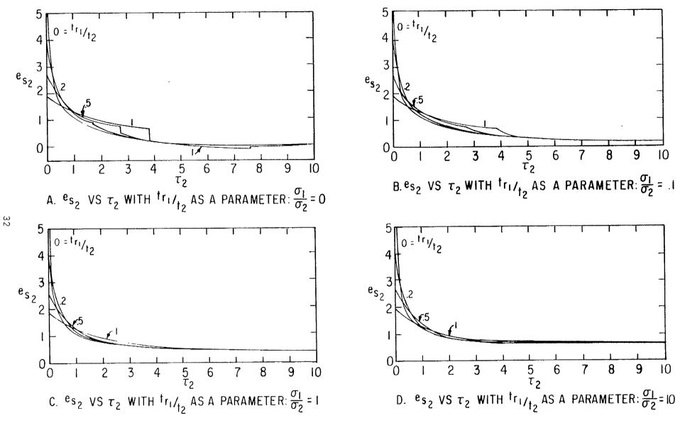
FIGURE 10. HORIZONTAL ELECTRIC FIELD PULSE SHAPE ON TRANSMISSION LINE:  $\epsilon_{r_1} = 10, \epsilon_{r_2} = 10, P_5 = 0$
