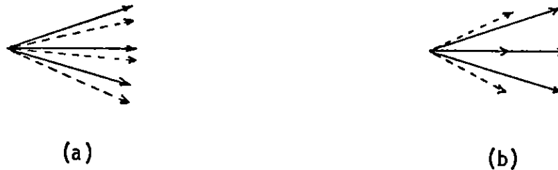
Figure (3) Change in momenta induced by a force, (a) perpendicular to \vec{p} , and (b) antiparallel to \vec{p} .
