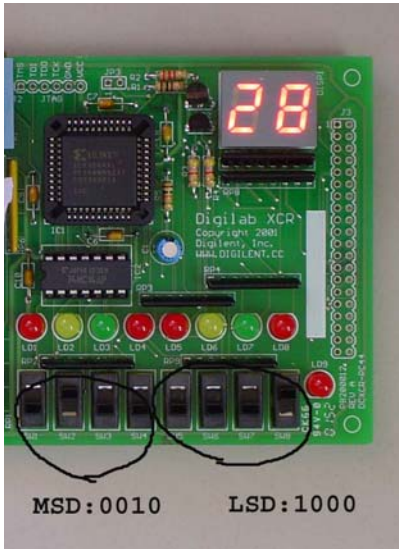
Figure 9; Display controller test
