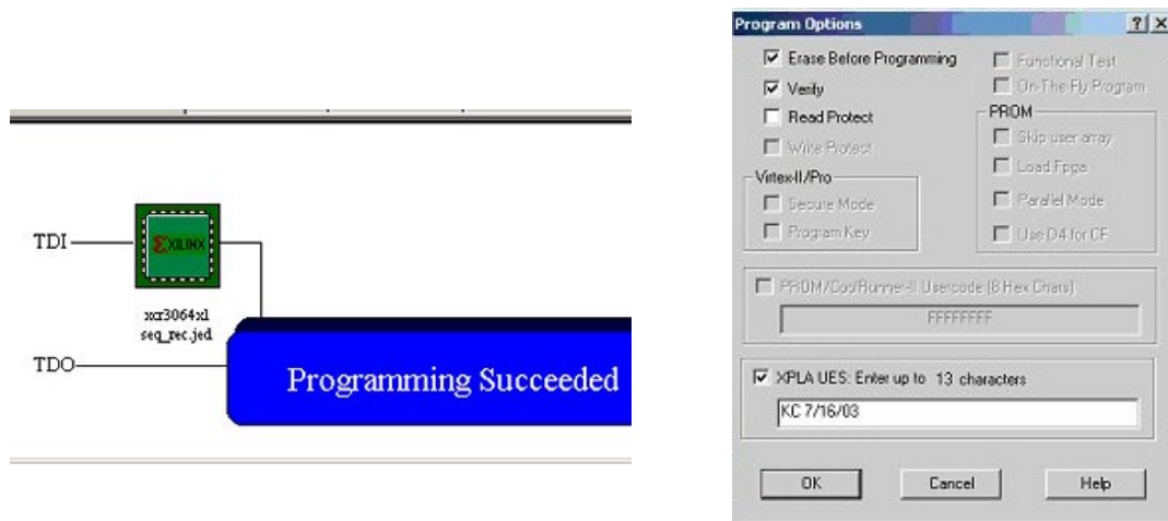
Figure 8; iMPACT window and options for CPLD configuration.
