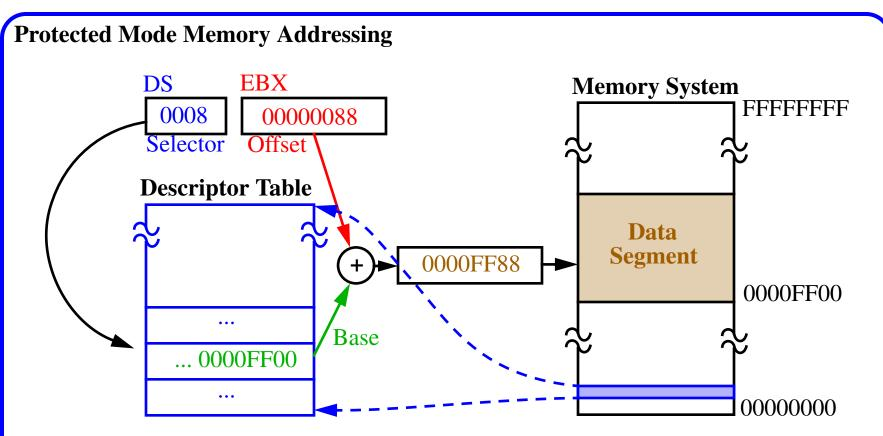
Segments are *interpreted* differently in Protected Mode vs. Real Mode:
