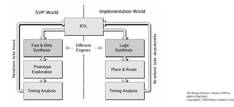
The gate-level netlist of the *SVP* is not as accurate as the final version.
