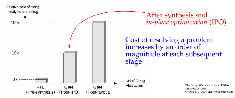
*Timing closure* refers to analyzing a design or architecture to detect and correct any problematic timing paths.
