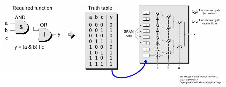
Input signals can be decoded using a hierarchy of *transmission-gate* MUXs.
