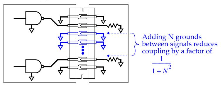
• Each of the wires in the connector couples noise, so simply reducing the number of signals in the connector cuts aggregate crosstalk. As shown above, you can create *virtual* partitions within the connector
