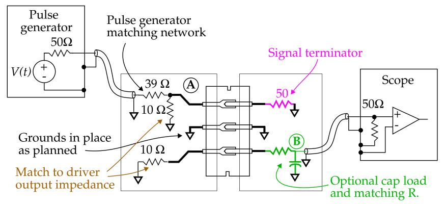
The pulse generator should be adjusted to produce a signal with a rise time similar to the driver that you'll use.
