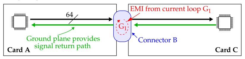
Connector B provides ground pins for signal return current.
