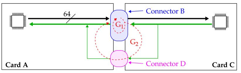
The proportion of high speed current that flows through connector D depends on the ratio of loop inductances.
