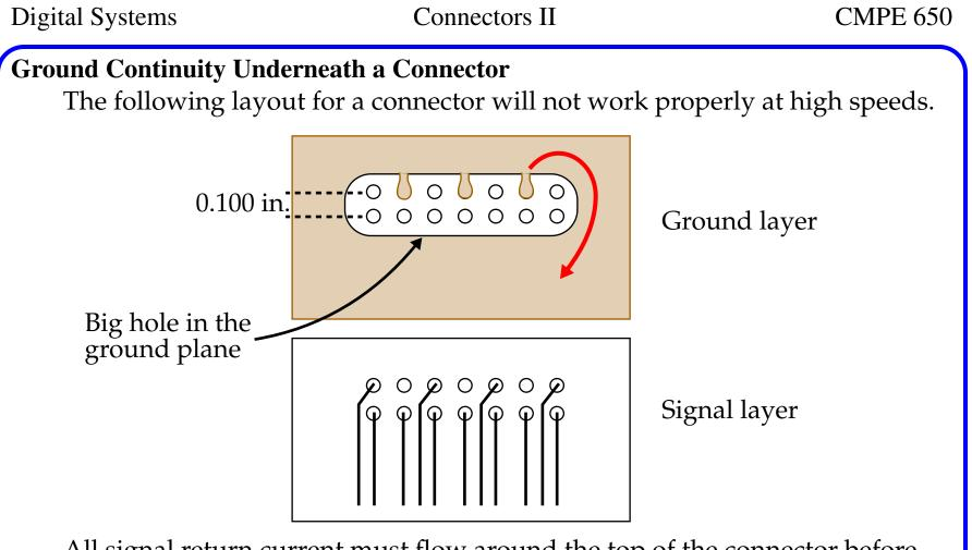
All signal return current must flow around the top of the connector before rejoining the signal path.
