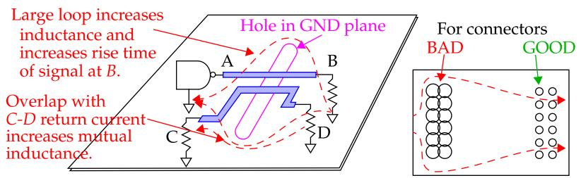
You may be tempted to do this when you run out of room on the regular routing layers and *cram* a trace in on the GND plane.
