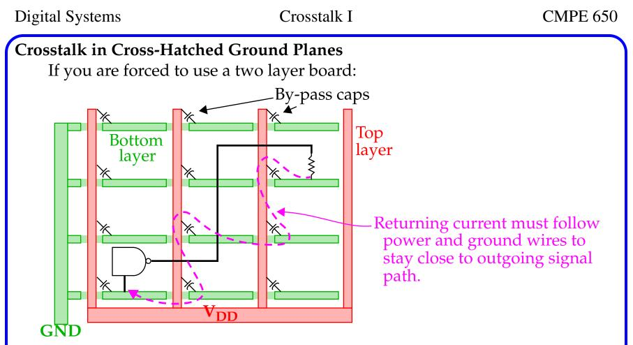
Note that signals are interleaved with the power and GND routing. This layout increases *mutual inductance*.
