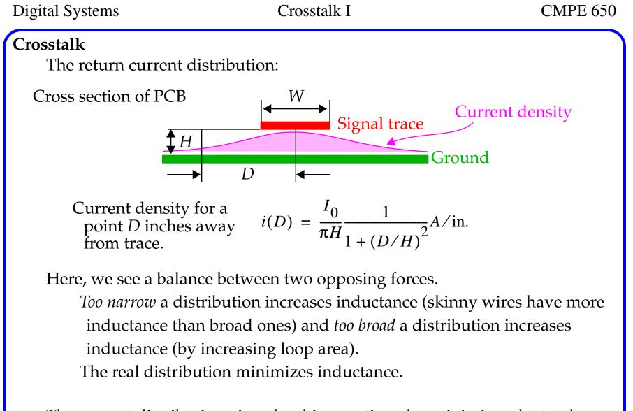
The current distribution given by this equation also minimizes the total energy stored in the magnetic field surrounding the signal wire.
