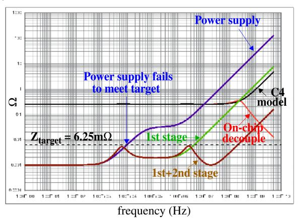
Note that both of these impedance profile plots include the effect of parasitic series resistance of the capacitors called **equivalent series resistance** or **ESR**.
