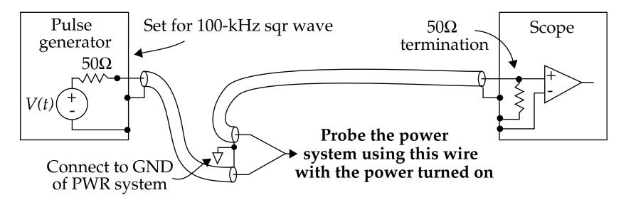
The output impedance of this arrangement is 25  $\Omega$  (parallel of 50  $\Omega$  from pulse and scope).
