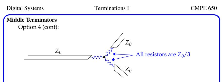
In this configuration, the signal attenuates by 1/2 as it passes through each juncture.
