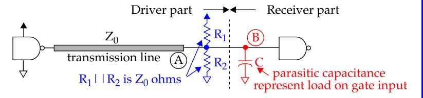
Here, the ratio  $R_1/R_2$  controls the relative proportion of *high* vs *low* current.
