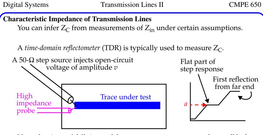
Here, the rise and fall times of the measurement setup complete well before one round-trip delay of the transmission line.
