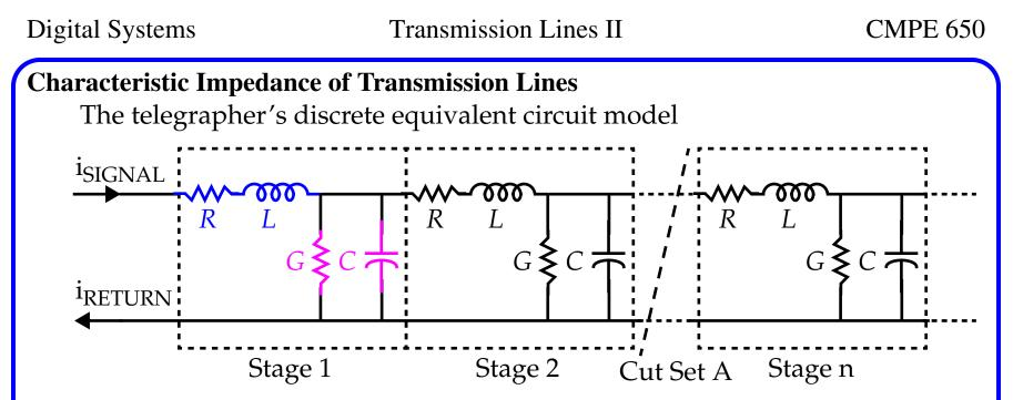
The series impedance *z* (R and L) and shunt admittance *y* (G and C) are *per unit length* of the transmission line (1 meter in our case).
