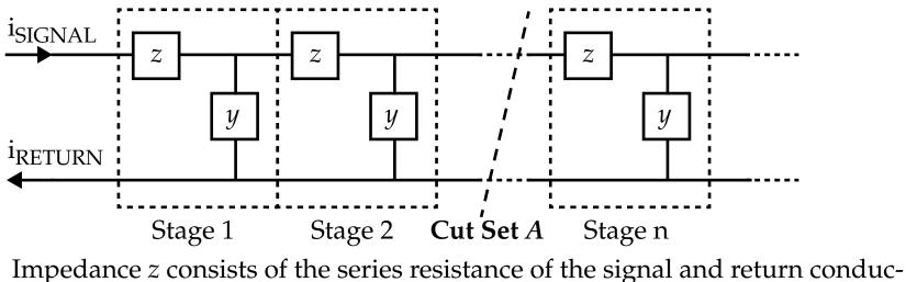
Impedance *z* consists of the series resistance of the signal and return conductors and inductance.
