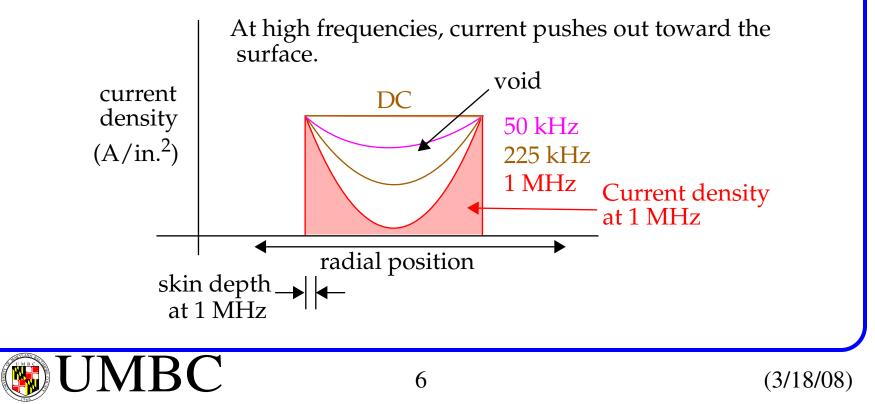
Assume wire is sliced horzontally into a series of concentric wires High frequency current follows the **path of least inductance**
