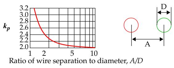
The same forces responsible for the proximity effect also cause ground plane return current to follow closely underneath a signal conductor.
