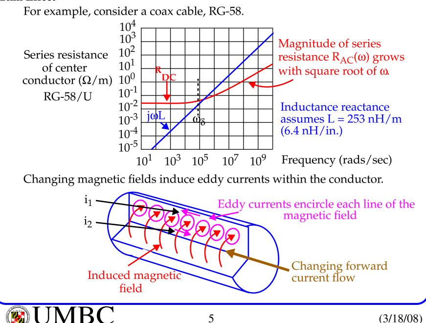
Note that the magnetic fields cut through the body of the conductor, and induce eddy currents, whose magnitudes are proportional to  $\omega$ .
