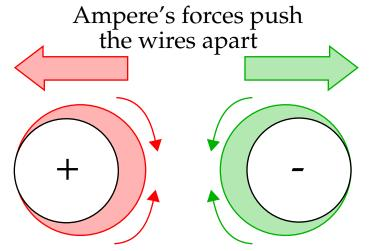
Proximity effect squeezes current together causing the highest current density at inside surfaces
