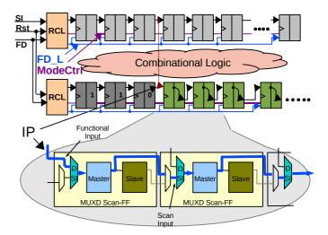
Fig. 1: REBEL embedded test structure.
