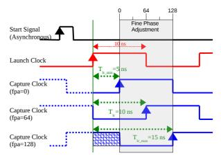
Fig. 3: Launch/Capture Timing Diagram
