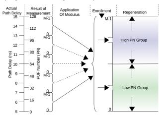
Fig. 4: Dual-PN Path Delay Binning Technique
