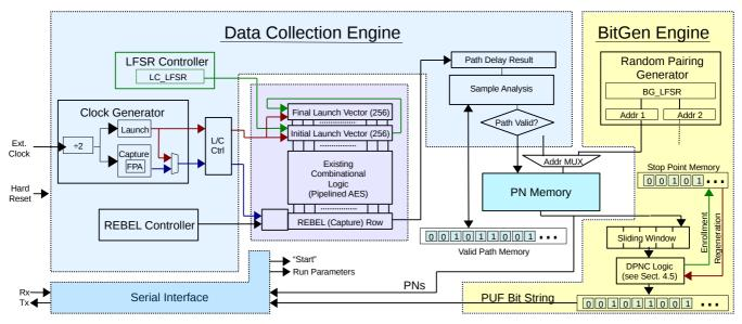
Fig. 2: Top-Level HELP System Diagram
