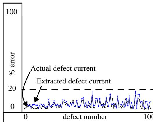
**Figure 12. Chip C3: Curve derived prediction results.**
