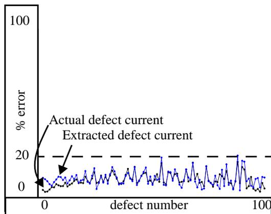
**Figure 11. Chip C3: Linear equation prediction results.**
