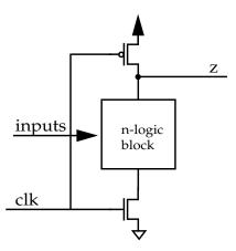
c) (8pts) Briefly explain how the following dynamic logic cir cuit can fail, using timing diagrams for clk, i<sub>1</sub> and z. How does CMOS domino logic solve this problem?
