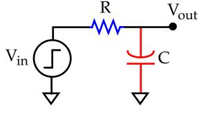
Step input produces an exponential transient response.
