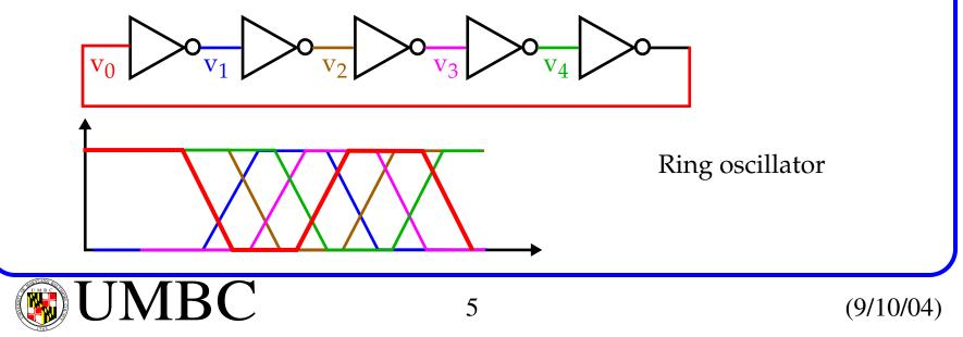
The ring oscillator is the *de-facto* standard circuit for **unbiased** delay measurements.
