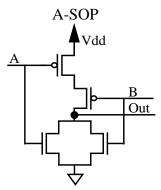
14) (4 pts) The single stuck-at fault model assumes exactly one fault is present in the circuit. Give the test for *C SA0* and show that it is not possible to detect it when *A SA1* is also present in the circuit. What is this called?
