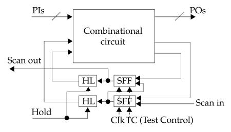
20) (6 pts) Launch-on-shift and launch-on-capture are two alternative strategies for performing delay test in a scan environment. Briefl yexplain how  $V_2$  is generated in each of these schemes.
