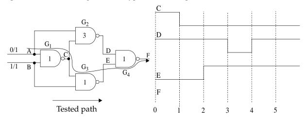
16) (4 pts) Is the test of path *A*-*C*-*E*-*F* in the above circuit *hazard-free robust, robust* or *non-robust*?
