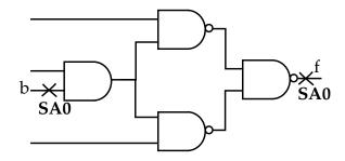
12) (6 pts) Equivalent fault collapsing has been applied to the following circuit and collapsed faults are indicated with an 'X'. Apply dominance fault collapsing and list the faults that remain!
